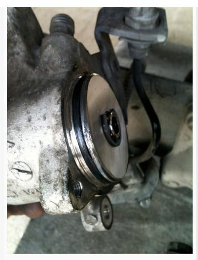
Same with the mating surface of the parking brake motor. This will ease the installation process and promote a good seal.
