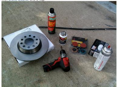
Next, put a non-directional swirl finish on the new rotors using the 3M Scotch-Brite ROLOC surfacing discs and a cordless drill.
