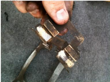
Lubricate the pad-contact points on the shims and reinstall.
