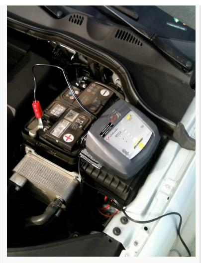
Pretty simple. This MUST be connected to prevent your battery from draining while you perform the brake job. (Ask me how I know) Yes - you need to leave the car ignition in the "ON" position (not running of course) to maintain comms between the VAGCOM and the car. Without a charger in place - the battery will die and trip just about every light and code possible (See "Uh-Oh" section)
