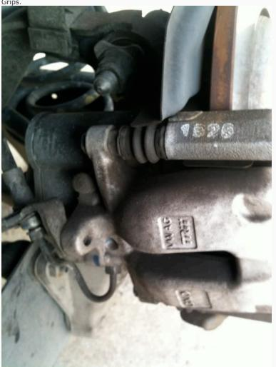
I didn't have a wrench thin enough to fit between the caliper and the bracket  $\mbox{-}$  so a vice grip was used in its place.
