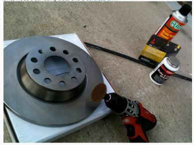
This non directional swirl finish helps to eliminate noises and aids in breaking-in the new pads.
