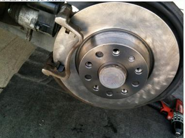
Snap in the new pads. I went with Wagner Thermo-Quiet Ceramic brake pads as they're quieter and produce less brake dust than semi-metallic pads.
