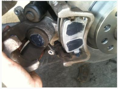
Reinstall the caliper. Ensure all bolts are tightened. Check the caliper slides. (see video - click the pic below)
