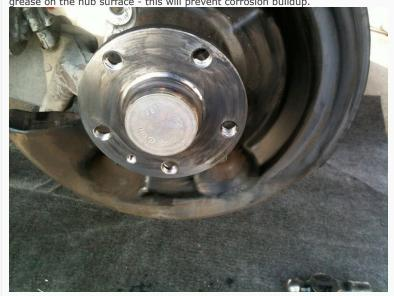
Install the new rotor. Secure it with the retaining screw.
