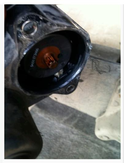
Put the electronic parking brake motor back on the caliper. It should go back together without any issues.
