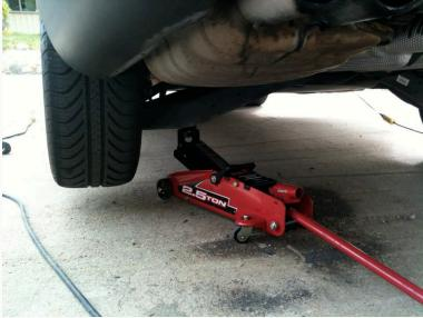
Place your jack stand on the pinch weld where your factory jack would normally be used and remove the tire. When you remove the jack, the control arm will travel down allowing you more room to work on the brakes.
