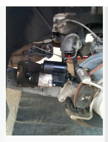
6. Remove the caliper bracket using the MT14 triple square socket.
