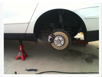
5. Remove the caliper using a 13mm socket and a pair of needle nose Vice-Grips.
