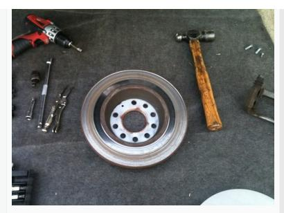
8. Prepare the new rotor for installation. New rotors usually come covered in packing oil to prevent corrosion while sitting on the shelf. Remove this oily film with Brake Cleaner and a rag.
