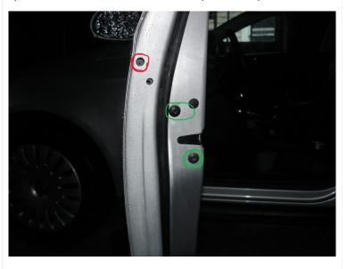
i) Remove the door lock bolts (2 M6 bolts)
