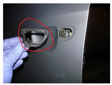
I) Make sure the door handle bracket is free from the door when you remove that "gasket" (red circle), and then pull the subframe up a little bit, tilt the bottom out, and pull it downwards out from the door frame.
