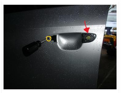
j) Remove screw circled in yellow (T20), and then pull of the door handle bracket "gasket" (red arrow). Pay attention to how it's installed. k) At this point you can remove all the bolts securing the subframe (subframe picture – yellow circles)
