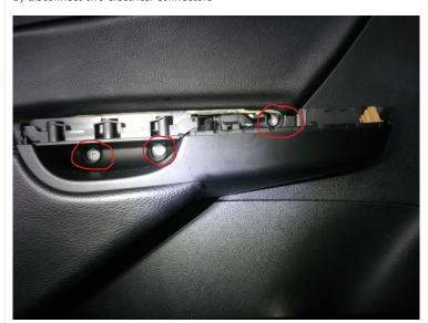
c) remove three T30 screws behind the door handle cover (red circles above), and two T20 screws at the bottom of the door panel trim (not shown) d) Now you need to pull the trim off the door. There are six clips holding the trim to the door – 3 on each side. I used a butterknife to find them, and then I pulled the door trim off the door.
