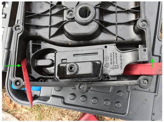
Be sure to pry with something that won't harm the plastic that the Valve Cover and Oil Separator are made of. I used nylon trim removal tools.
