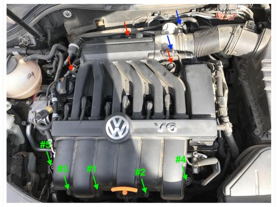
Once you're done with that, remove the two vacuum hoses from the back of the manifold, marked by the blue arrows:
