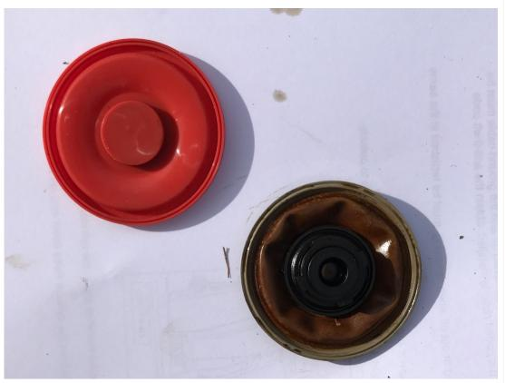
RKXTech's is made out of a much thicker material. This shouldn't cause problems as the valve's response is controlled by the springs on either side.
