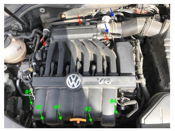
First unbolt the fuel line bracket directly in front of the oil fill cap. It attaches to the Valve Cover with two T30 screws.
