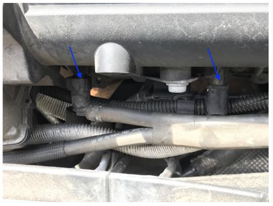
The one on the right in this photo (passenger's side) is a snap-on compression connection. The other one uses the same clip that VW uses on fuel lines. To remove it, press in on the white-ish clip and pull out:
