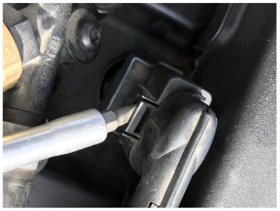
Next, unclip the tray holding the coil harness from the intake manifold. It's held in by three "Christmas tree" clips which come out with firm but judicious pressure:
