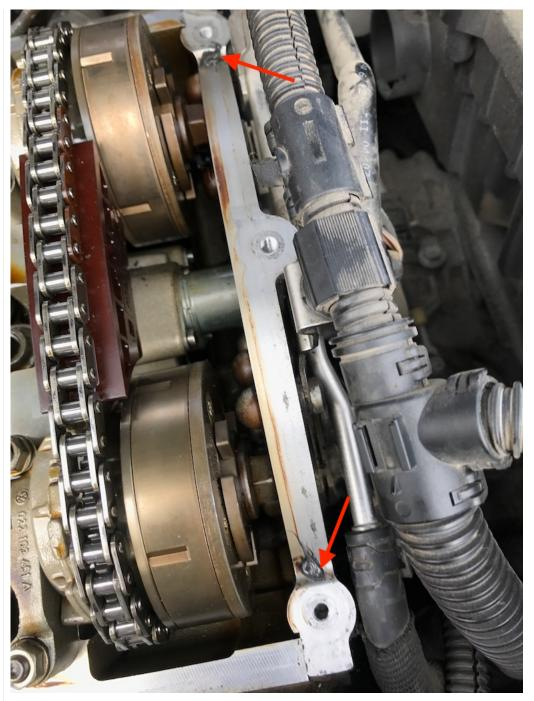
Set the Valve Cover into place and tighten the bolts to 10Nm, in sequence, in steps. I went finger tight, 5Nm, 10Nm. Here's the sequence again:
