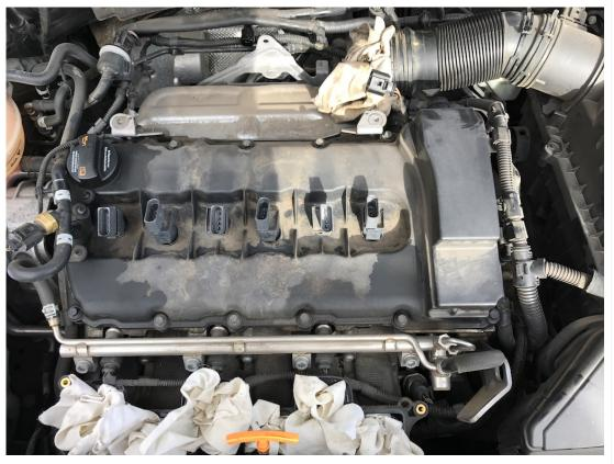
VW says a special tool is required, but with the manifold out of the way all you need is your hands. The spark plugs can remain as they are threaded into the head.
