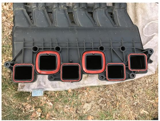
Set the manifold back in place. Tighten the bolts to the lower manifold in the order shown, again going finger tight, 5Nm, then 10Nm:
