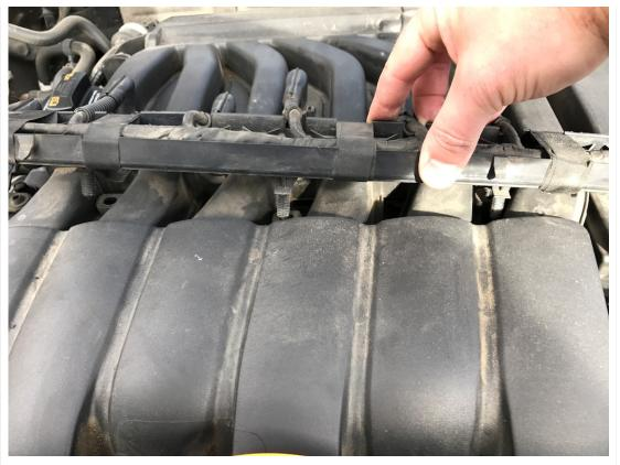
Set the tray to the right, over the air box. Next you need to unplug the electrical connections marked by the arrows in blue:
