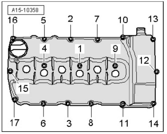
I loosened them in the same manner as the manifold bolts: break then loose, loosen 1/2 turn, loosen 1 full turn, and then take them all out.
