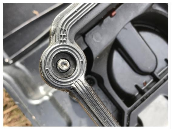
I put a light coat of fresh engine oil on the gasket with my finger.
