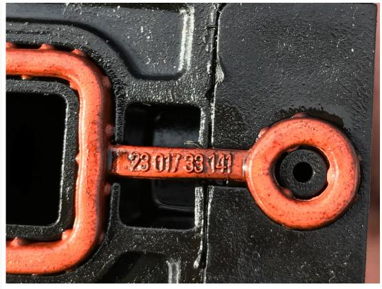
The diaphragm valve is inside the disc-shaped area right behind the gasket. I was able to pry it open by using a putty knife to work my way around the lid. Here's what you'll find inside:
