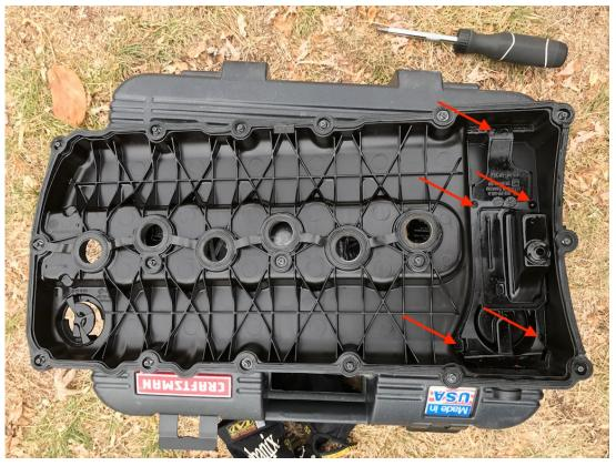
Even with the screws removed the sucker is going to be pretty well stuck in there. In theory you remove it by pulling straight up and out, but the gasket at the front of the Valve Cover won't want to let go.
