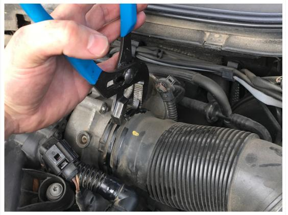
Stuff the throttle body pipe and exposed intake manifold runners with clean rags, and you're ready to pull out the coils:
