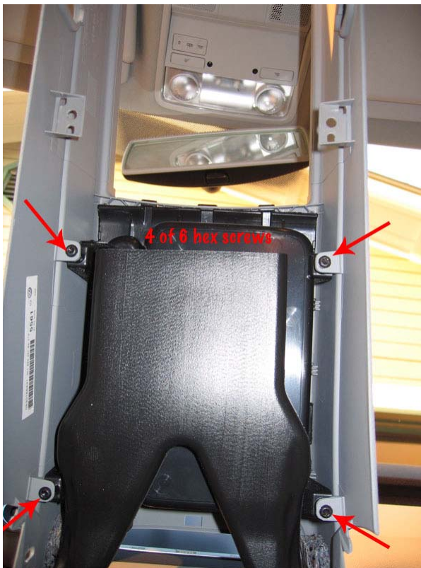
3.3 Unscrew the six hex screws holding the U.S. cupholder in place and replace with the European cupholder.
