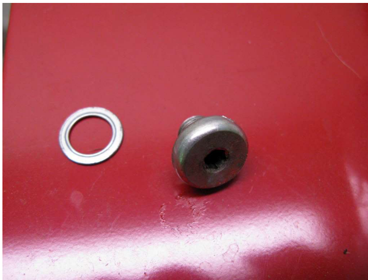
Drain plug removed, showing allen portion of ATF level tube:
