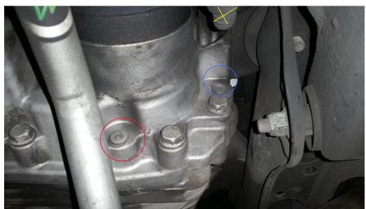
Cases can be filled using a gear oil pump. Best not to mix oils so get a few of em; inexpensive pumps from harbor freight tools do a good job. Haldex oil is pretty thick, so shake up the bottle (additives collect in the bottom) and heat it up a little to get it flowing.
