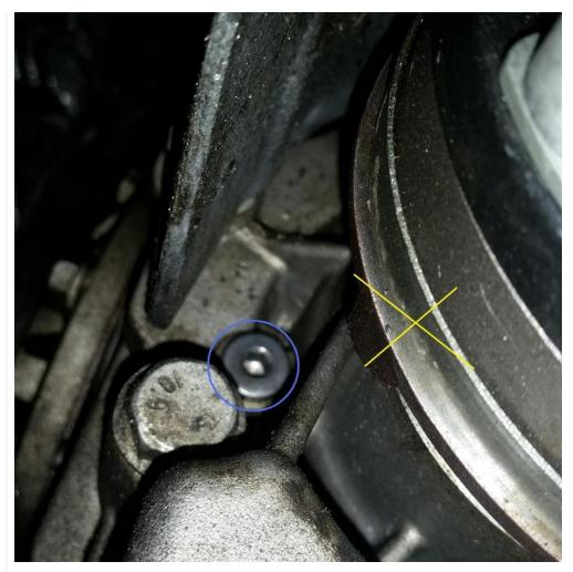
Side view of fill plug from r/f driveshaft:
