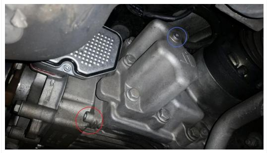
Fill til it spills, drive around to warm up oil. As per repair manual, "The oil temperature must be 20 to 40 °C (68 to 104 °F)" This is found in AWD electronics control module address 22, measured value block for control module temperature or clutch temperature; best to look at both. When warm enough and vehicle level, remove fill plug, let excess drain out to bottom of hole or as much as 3mm below fill hole.
