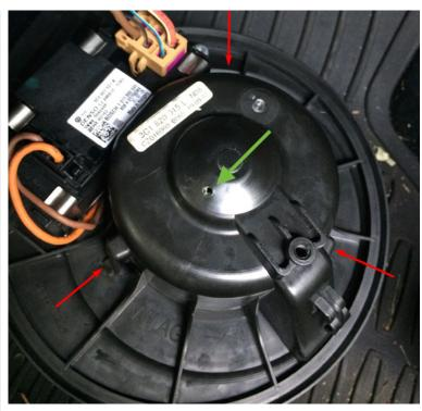
In the arrow marked places there are 3 rubber dampers to reduce vibrations, if you push them inside while pulling the motor from the plastic cover (they act like clamps) you can take it apart and do a better job at cleaning/greasing the bearings
