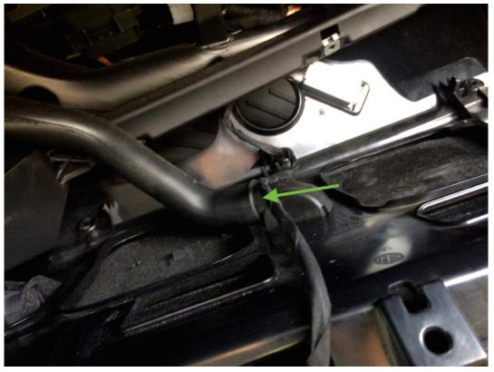
Next, unplug all the electrical connections (green arrows) and pop out the plastic wire anchors (red arrows) using the thin plastic crowbar with a notch in the end from your trim tool kit:
