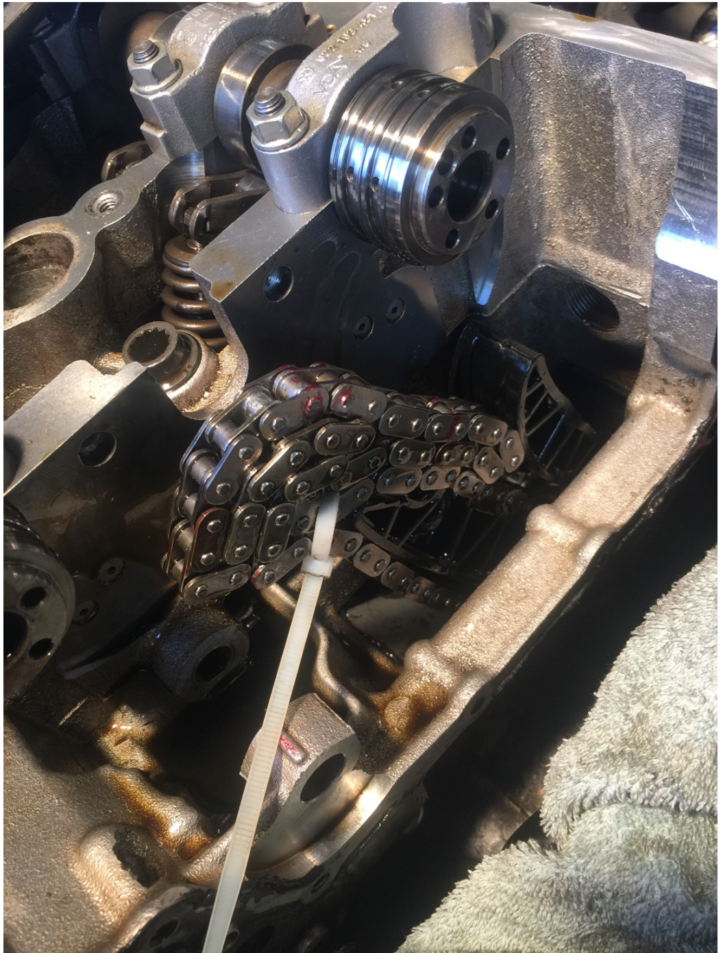
Without the sprockets on the cams cover them so no debris gets in. Ziplock bags with zip ties work great!
