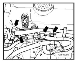
Remove intake manifold to the cylinder head securing bolts -arrows- with socket TORX® T30 -T10347- .
