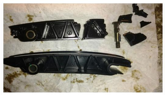
As you can see, the post that should have been covered by the chain guide was being worn away by the chain. I believe that this is what was causing my P0016 codes.
