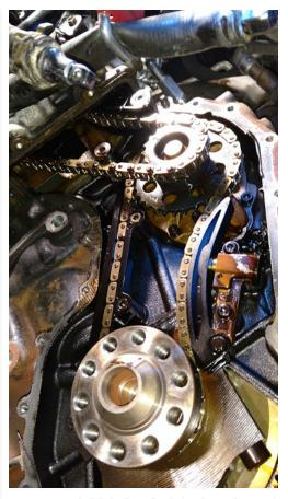
As you can see, the bolt (8.8) is still tight, but the top chain was loose. When I looked closer, I realized that the top chain guide was partially gone, and pieces of it were on the sides of the lower chain:
