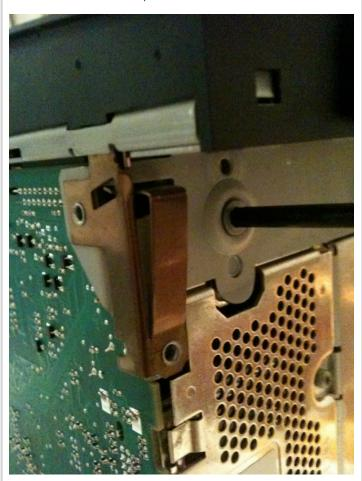
Now the fun begins. On the sides of the RN S2, you will see 4 large #20 torx screws (2 on driver's side, 2 on pass). Unscrew them. These screws screw into 4 sort of ledges, leaves or tabs coming from the front of the unit. Insert a flat screwdriver between such tabs and the main body of the RN S2, so as to "open" them or reduce the amount of pressure between them
