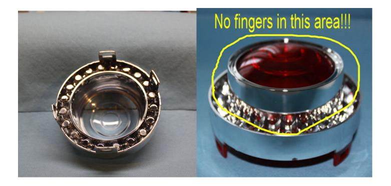
Drill out the holes for the LEDs, I used a 3/16" drill bit. Use compressed air to blow off the plastic garbage. Mount the LED board onto the back of the chrome ring. I used two small pieces of tape to hold it in place. Place the wires so that you can feed them through one of the holes in the back of the light (not the centre one!).
