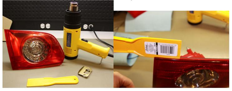
Next I suspended it upside down over two blocks so that you can press the four latches and pop out the center chrome ring. (Do Not touch the chrome!! You will not be able to remove the fingerprints without scratching the very thin layer of chrome)
