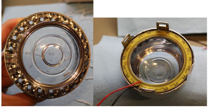
Feed the wire through your chosen hole and carefully insert the centre ring into the light. I used a blue lint free shop towel to push it back in. Don't touch the chrome with your fingers!
