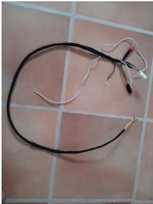
Now back to the car. Grab the 8K0972994 connector and insert the pins from the harness you just made, into it and snap it closed. Please make sure you insert the correct pins into the correct spots, if you don't bad thing could happen.
