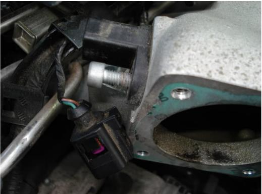
8.) Take electronics cleaner of choice, and spray the sensor down thoroughly. Be gentle with this sensor as it is exposed and wouldnt take much to mess up the small wires running through it. Make sure it is good and dry, and re-install.
