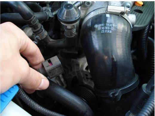
4.) Loosen the hose clamp holding the Throttle body hose to the actual throttle body, and gently wiggle the hose off the end of the TB. If its giving you a hard time, slowly turn it back and forth a bit, GENTLY, while pulling, it should come right off.
