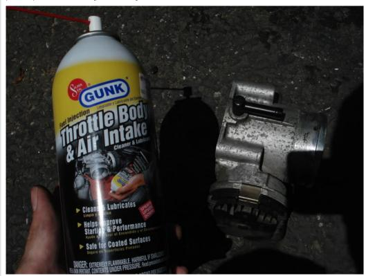
Be careful when cleaning around the butterfly valve as it is a precision piece, it only "tilts" or turns one way, so be sure not to force it to move. it will have a little resistance to get it to open, but dont go he-man on the thing. Clean around the small opening inside by opening the valve and get all that carbon out!
