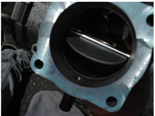
You can also remove the butterfly valve/throttle plate with a T20 torx driver and removing the 2 bolts holding it, for a more in-depth cleaning. I chose not to as it was not necessary and I was able to get practically all the build-up out, without a problem.
