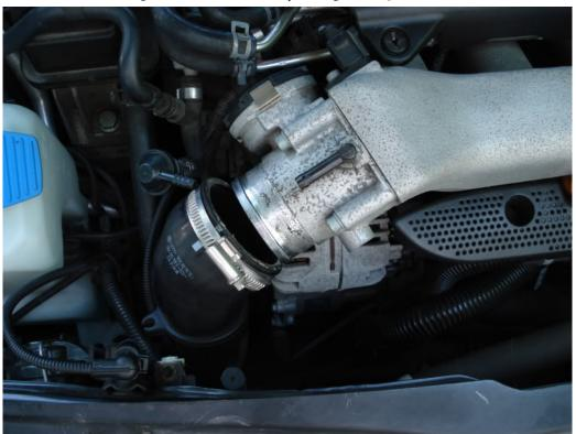
5.) At this point you can see inside the TB, and are getting closer to actually cleaning it. There will be 4 Allen bolts holding the TB to your intake manifold, they are 5mm. undo these 4 bolts and carefully release the TB from the intake.
