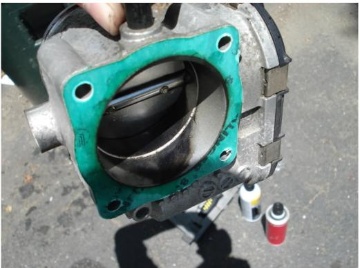
BE CAREFUL as there is a gasket between the TB and intake manifold that you dont want to damage/drop/bend. Mine was stuck to the TB itself, you can reuse this gasket or get a new one, your choice. (I chose to re-use mine as it was in decent condition) Just be sure to keep it clean and flat if you plan on re-using it.
