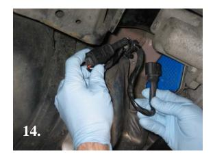
\*Zip tie and make sure that the harness is out of harms way. (drive shaft, heat shields, etc.)
