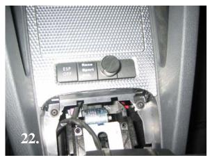
**Step 9:** Now remove the plastic blank and use a 31/64" drill bit to drill a hole for the selector.
