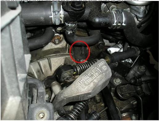
Remove the timing plug on the transmission so that you can visibly see the flywheel TDC mark. The Plug is located here.
