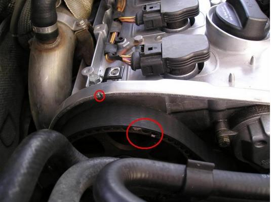
^ Here is where the cam gear lines up with the valve cover. You can also see the mark on my cam gear and my new belt from the nail polish. They don't line up because the car has been running.
