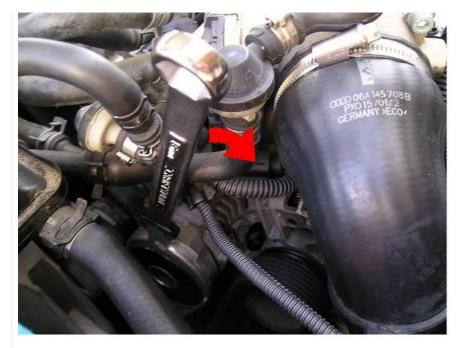
Now the accessory belt tensioner is locked in place and you can easily remove the belt. Then remove the intake pipe to the throttle body hose. When finished with all that, use your ratcheting 13mm wrench to remove the accessory belt tensioner and place that out of the way.
