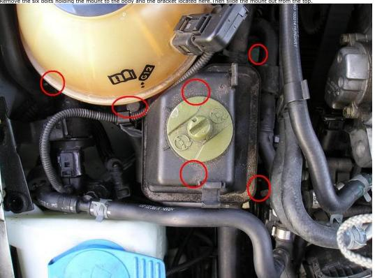
Remove the six bolts holding the mount to the body and the bracket located here. Then slide the mount out from the top
