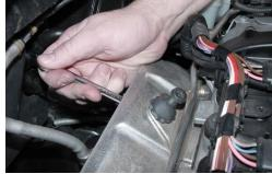
Installing NEUSPEED heat shield: First remove the (2) 10mm hex nuts located on bottom side of factory heat shield connecting the rear air filter box (engine cover) mounts. Then using a 24mm 12 point socket, unscrew the mounts.
