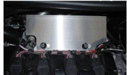
7. Install NEUSPEED heat shield using original air filter box mounts with SS washers supplied. Then reinstall 10mm hex nuts on bottom side.
