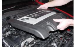
There are four rubber grommet mounts holding air filter box (engine cover) to engine. Lift up one corner of air filter box at a time to detach.
