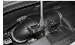
Unclip and disconnect turbo intake hose from air filter box.
