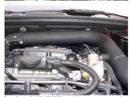
9. Install NEUSPEED intake pipe onto turbo inlet with #40 clamp supplied and attach rubber isolator mount to ear on end of cylinder head with M6x10mm screw. Intake pipe should be positioned at an upward angle toward brake fluid reservoir for engine torque clearance, now tighten hose clamp and M6 screw. NOTE: When tightening isolator mount, do not over tighten – rubber isolator should not have any twisting force applied to it.
