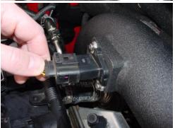
Install MAF sensor (fits one direction only) and tighten with two M4x8mm Philips head screws supplied. Attach electrical connector.
