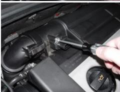
Disconnect electrical connector at MAF (Mass Air Flow) sensor and remove sensor mounting screws (T20 Torx), now pull out sensor.
