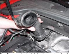
5. Remove turbo intake hose at turbo by squeezing spring clamp with spring clamp pliers. CAUTION: Do not let any debris or objects fall into turbo inlet or damage may occur.
