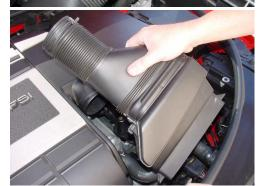
Remove the intake air duct: There are two T20 Torx screws that attach duct to the front core and a spring clamp at hose connection to the air filter box (engine cover).
