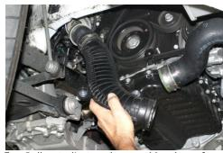
5. Pull-out clip to release rubber hose from turbo discharge.
