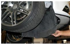
Undo the (8) T25 Torx screws to remove lower engine pan. Now remove the passenger side lower inner fender liner there are (5) T25 Torx in the fender well and (2) T25 Torx on the bottom of the front bumper cap. **NOTE:** Some models may vary slightly.
