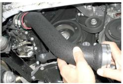
10. Loosely install second #36 hose clamp onto silicone hose. Now connect NEUSPEED discharge pipe to silicone hose and attach mounting points to engine. First tighten mounting screws then tighten second hose clamp.
