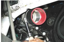
8. Install and tighten silicone hose to adapter using supplied #36 clamp.
