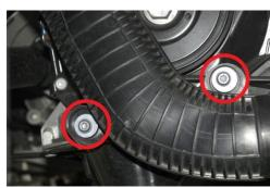
4. Unbolt plastic pipe from engine just below crankshaft pulley, (2) T30 Torx.
