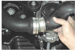
11. Again, lightly oil O-ring on intercooler hose and then install into NEUSPEED discharge pipe making sure it locks into place.
