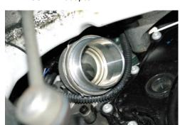
7. Lightly oil O-ring and install adapter into turbo making sure it locks into place.
