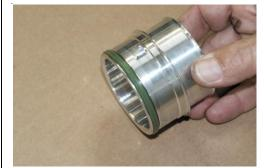
Carefully remove O-ring seal from original discharge hose and install onto NEUSPEED adapter.
