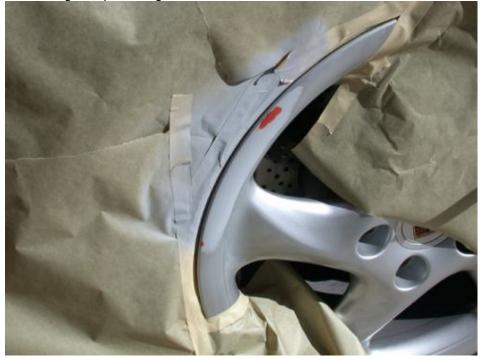
Okay, here's where a bit of laziness is going to create an entire new clay-bar project. This metallic paint will GET EVERYWHERE. I'm talking permanently attached to the fender on the opposite corner of the car...mask CAREFULLY and COVER THE WHOLE CAR with a sheet or equivalent.
