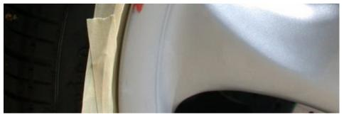
I like to START by masking the tire from the wheel...get the masking tape WELL behind the rim. Next, sand the area to a nice "feather" with 240 grit sandpaper and wipe some spot putty on. IMPORTANT...this ENTIRE project will work best if the wheel is in the sun and its a nice warm day...the drying time of spot putty is minutes but if it's cold or damp, this project is likely to not work out too well. Remember...keep your sanding to the IMMEDIATE area around the damage. Trust me on this.
