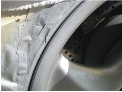
okay, fast forward a few minutes...I had to roll the car forward a bit to keep it in the sun and I had cleaned (and let fully dry) the wheel and RE-sprayed the silver. Now I'm using the NASA technique on the silver paint and CAREFULLY removing the overspray:
