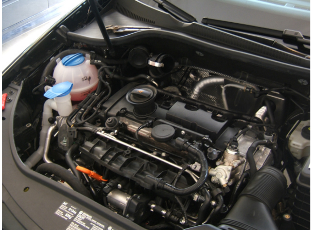
Step 2 - Take off the noise pipe thats on the passanger side of the engine cover.
