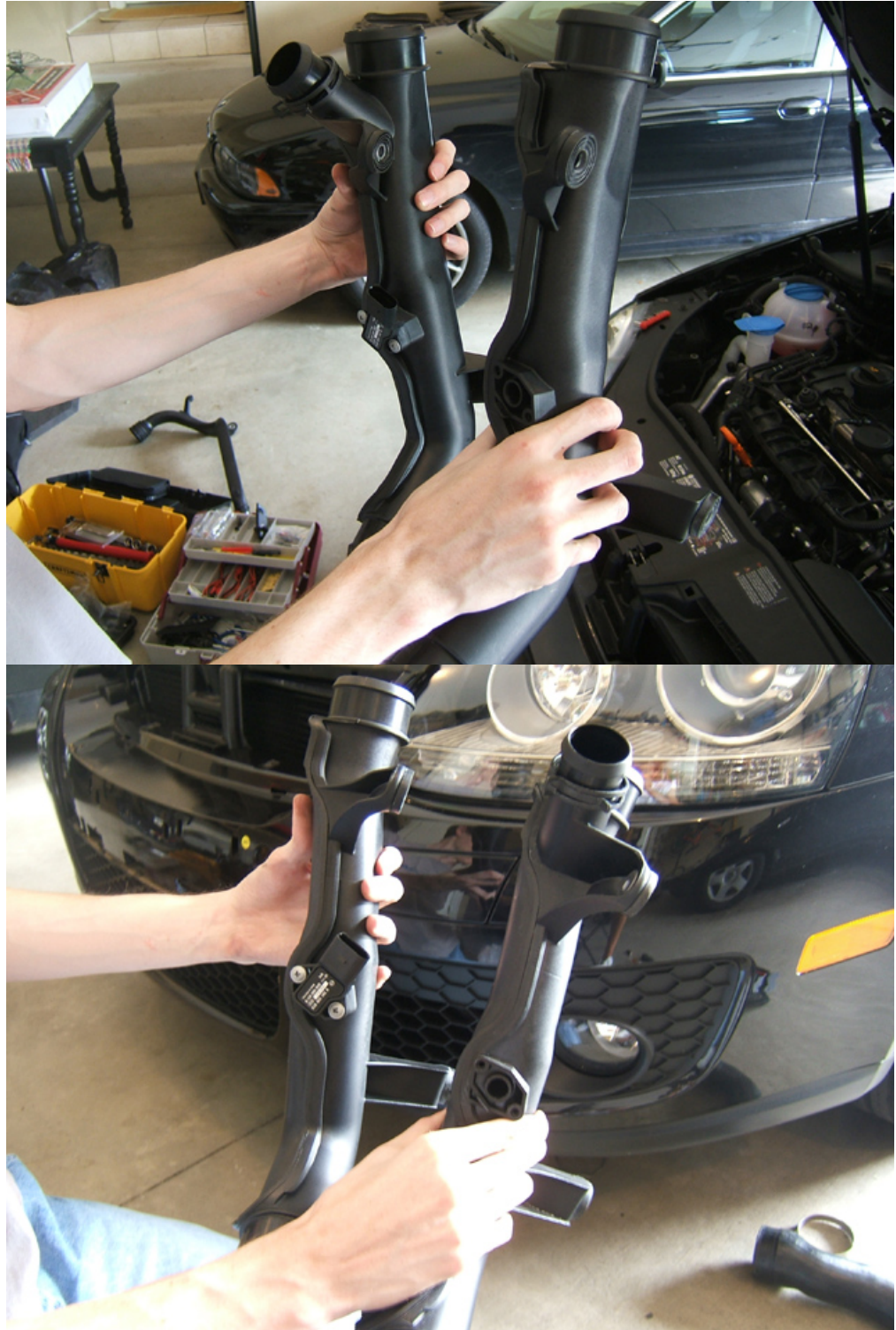
Step 1 - Take off the MAF Sensor and the Engine Cover
