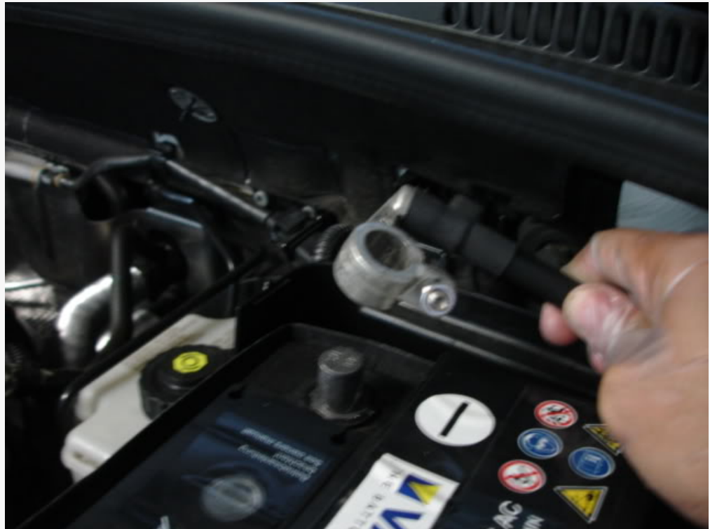
Unscrew positive Terminal using the 10mm ratchet and remove wire:
