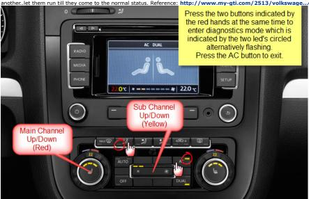
nd Step :Compresor Settings: Starting the engine and hold LONG-AC + heating rear window.Let it run till it comes to the normal status.
