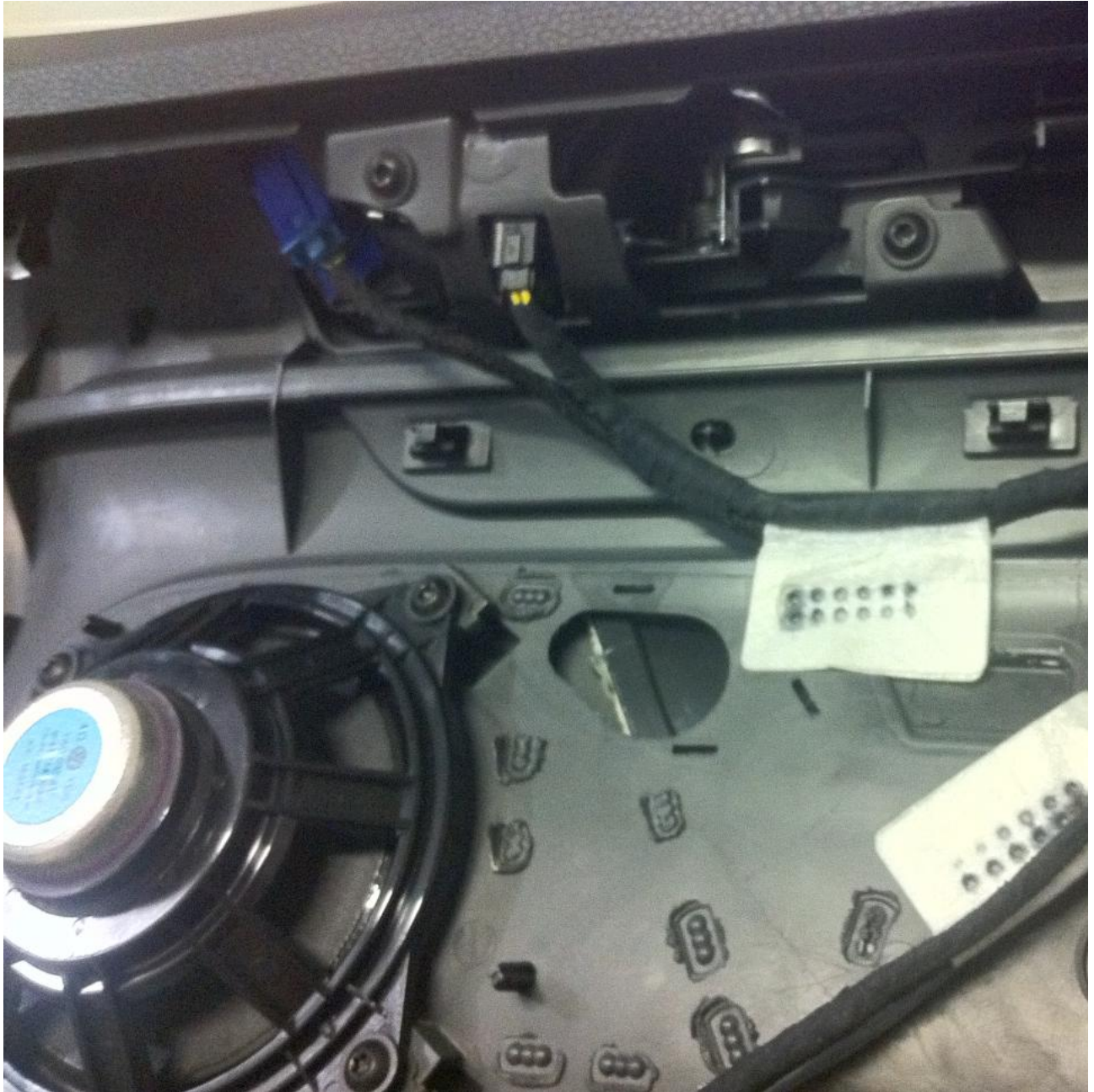
This is the intire wire leads all wired and tape up to the door card wiring harness for OEM install.
