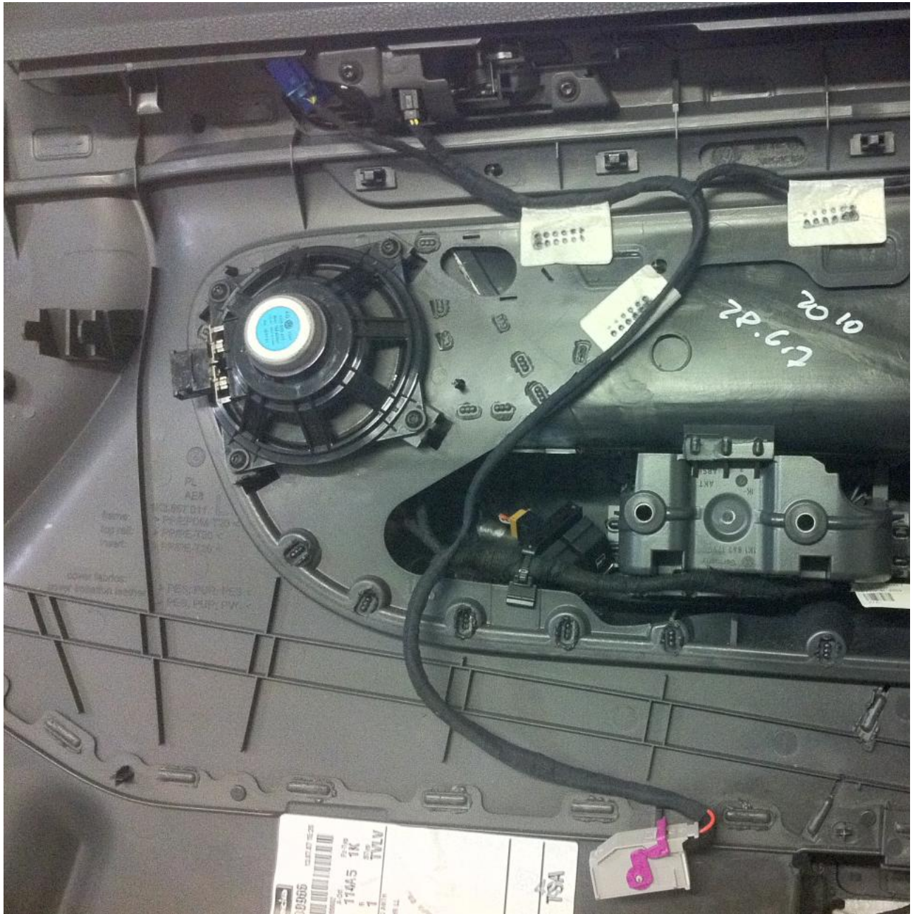
Close up the door card wiring harness with 32 pin connector, I wired the power wire to pin 26 and the negative/ground wire to pin 21
