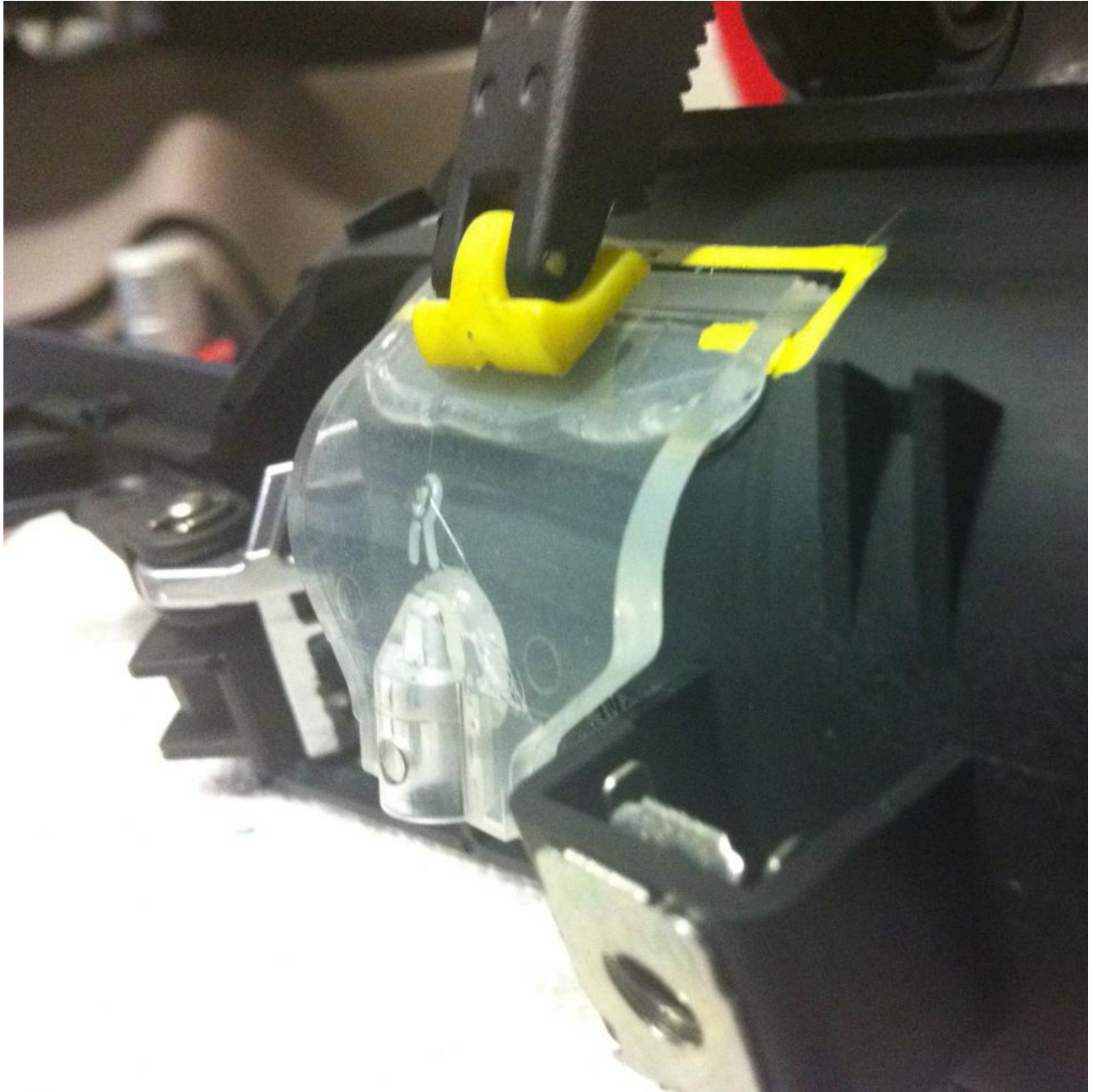
Close up of the back door handle installed and wire up and lead wires taped to door wire harness for OEM installation.
