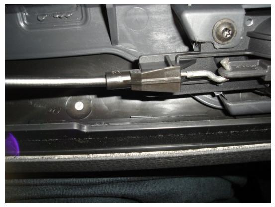
Now Disconnect the mid speaker connector (not pictured as mine is wired differently now) and disconnect the control cable by lifting up on the latch and pulling straight out.
