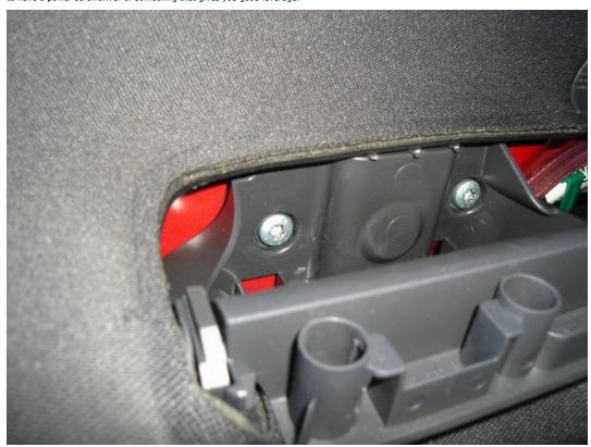
Once those are off there are 4 other torx screws. One is by the tweeter, the other 3 are at the bottom of the door panel. Use a T-20 bit to remove these.
