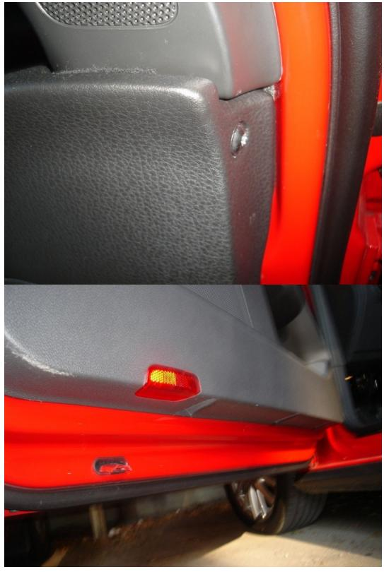
Now that the screws are out its time to remove the door. Best way to do this is to start near the front of the door where you can grab onto the panel. Pull straight back and the 2 forward fasteners should come loose. Then pull from the rear end and that should release the other 3 fasteners. Then just pull straight up to lift the door off. The top seal may stay connected to the door which is fine.
