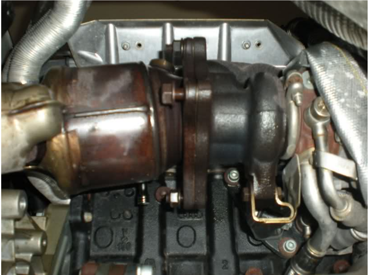
The worst bolt to get off, I used a stubby socket and reached hand up there, left socket hanging from it for pic purposes :)
