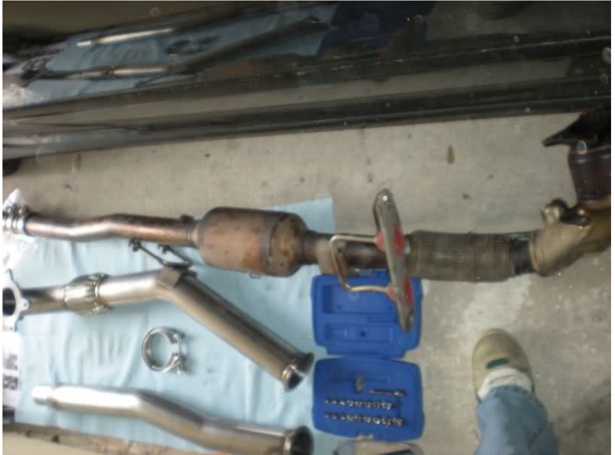
Stock dp mount attached and dp bolted on
