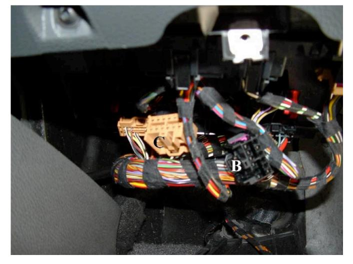
Now, insert the Grey/White wire you just removed into connector B in position B4. Remember to release the pink locking clip before trying to insert the wire.
