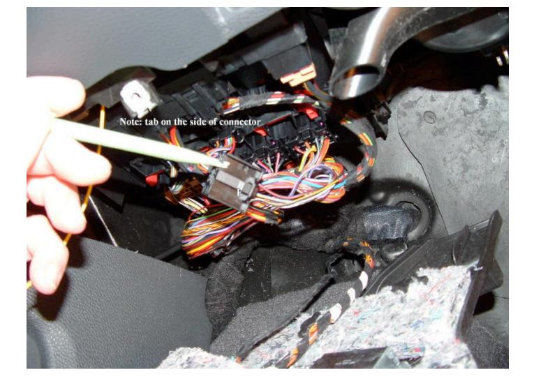
Pull out the E connector. You will notice it has a shell similar to the one on the headlight switch harness. This is because this is the other end of the headlight switch harness.
