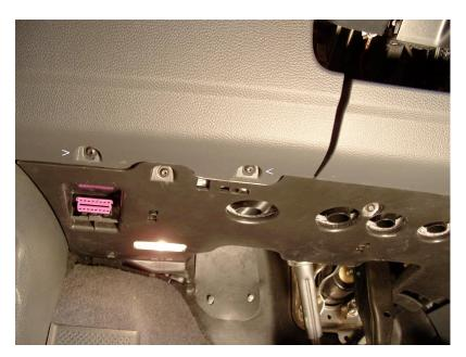
First remove the two torx screws from the under dash cover.
