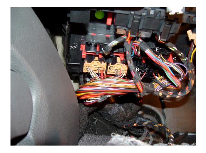
Here is the ECU we're going to be dealing with. The three connectors we're concerned with are labeled B, C, and E in the above picture. The arrows are pointing at the master un-locking mechanism to release the locks on the connectors. Slide it towards the drivers side to unlock it and to the passenger side to lock it.
