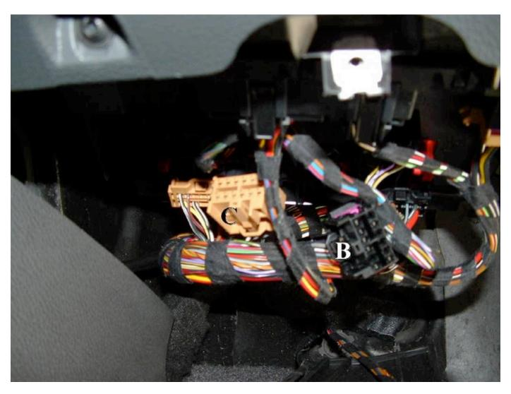
Disconnect connectors B and C from the ECU the same way you released connector E. Remove the pink retaining clips from both connectors using the small screwdriver to gently pry on the large side of it.
