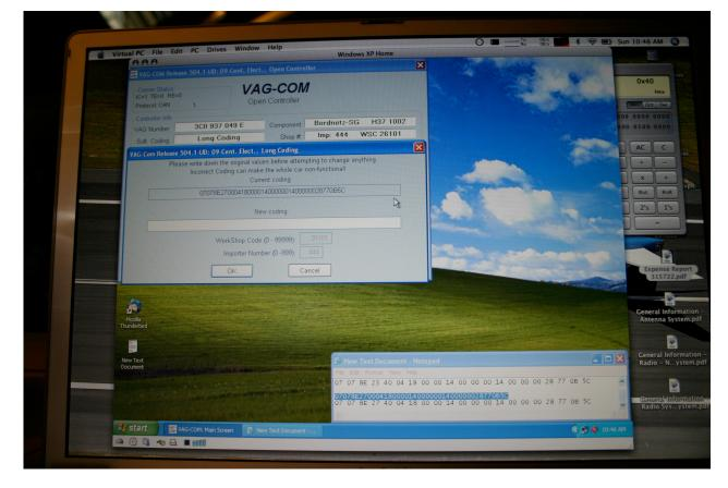
Using VAG-COM you will need to change the following settings in control module 9 (Central Electronics):
