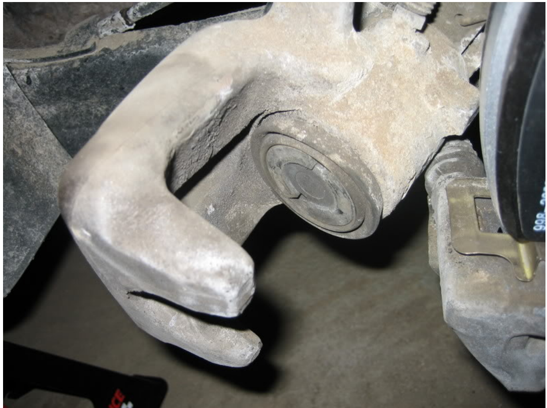
Your pads should have come with new guide pin bolts, VW suggests that you replace these when you put in new pads. Mount up your caliper.
