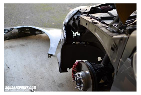
To reinstall your fender is basically the reversal of this process, though I recommend sliding the fenders back into the bumper mount before you start bolting things down. Also, be careful not to over tighten any of the bolts during reinstallation..
