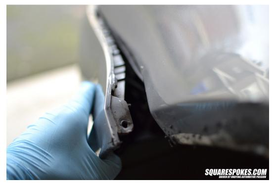
Now to the easy part. locate the remaining bolts holding the fender..
