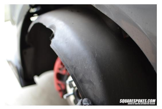
Once the fender liner is removed, locate the bumper / fender alignment screw on the edge of the fender..
