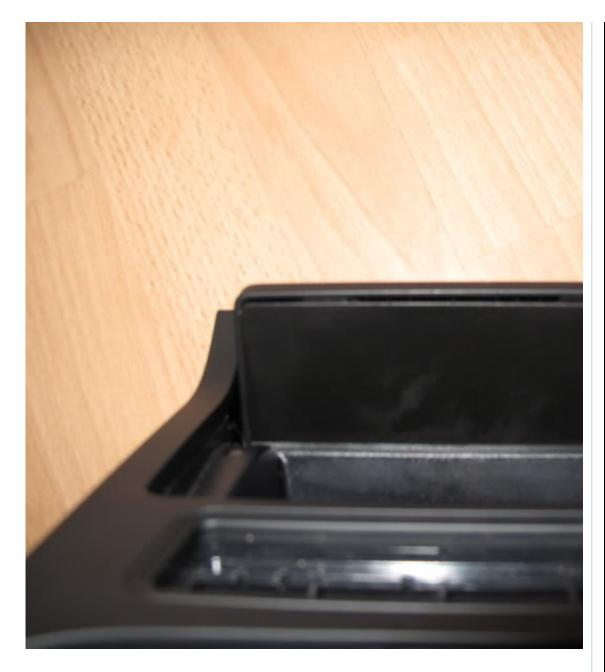
Now the hard bit, at the back of the ashtray is two more clips but there much harder to reach as there enclosed in the base, you will need to access the clips from two holes in the bottom, when they are popped of theres just two little clips in the middle of the lid and gentle force should remove these.
