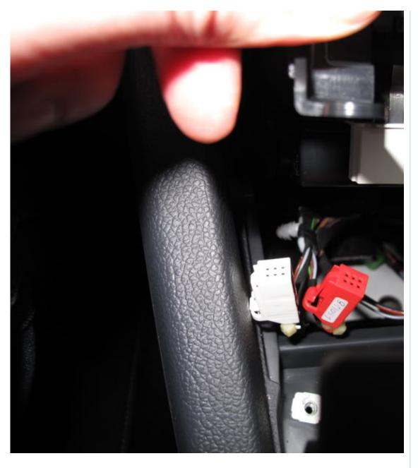
Then the ashtray will just slide backwards out of the hole (this is why you need to select 4th gear to allow its removal)
