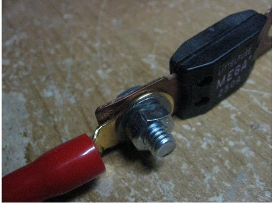
Attach the fuse to the bus bar:
