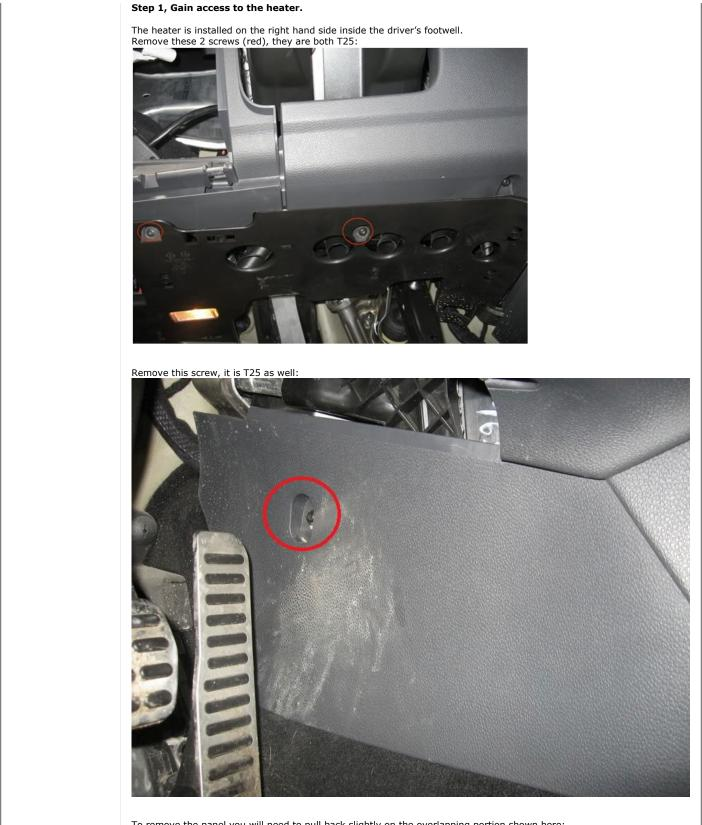
To remove the panel you will need to pull back slightly on the overlapping portion shown here:
