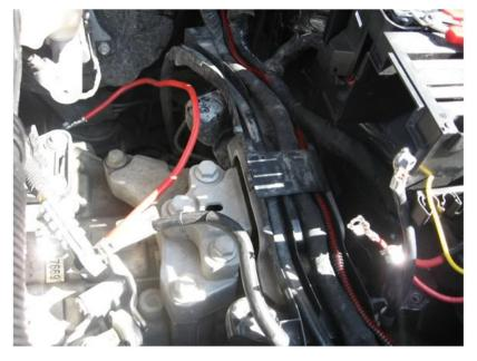
Step 3, Attach positive wire to the bus bar:
