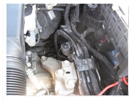
Step 2, Pull wire through firewall: This is the rubber gasket where the wire will come out of. Simply pull on it till you just enough slack on the inside to make the wires neat:
