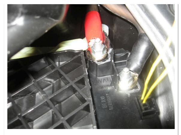
In the above picture the cover has been reattached. The red line is where I trimmed off the plastic where the cover is now. The 3 remaining bolts were used to attach the cover. Here is the piece I trimmed off:
