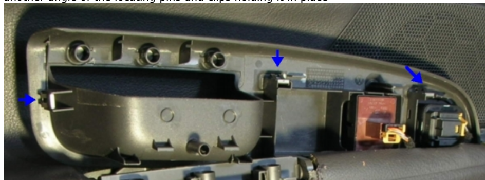
another angle of the locating pins and clips holding it in place
