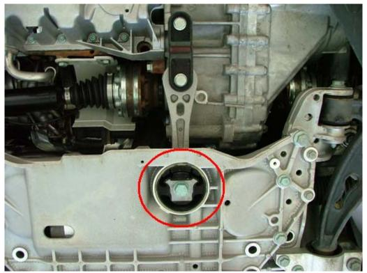
Locate and remove the bolt indicated in the picture. (21mm)
