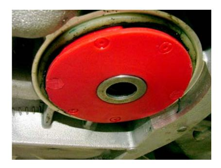
Insert the washer in the center of the insert.
