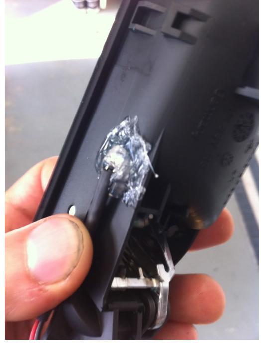
6) I used CAT5 cable twisted pairs, but you can use any wire really. You just need a pair for each **door** (ground and power). Strip the which one goes to ground and power, solder them to the LED power leads.
