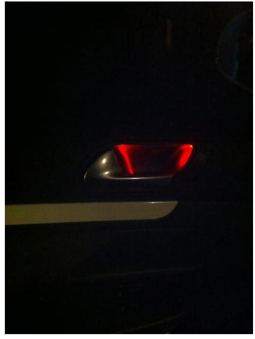
These only come on when the dome light is ON and the key is NOT in the ignition. So when I stop and turn the car off, they turn on. I approaching the vehicle, unlock the car, open the **door** and get in, they are on until I put the key in. This is also how my **door** warnir work as well. Footwell lights are just on whenever the dome light is on (does not depend on the key).
