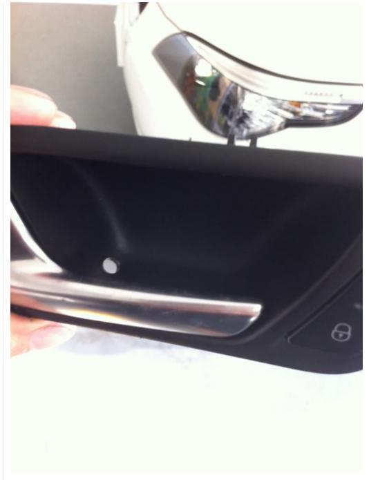
The hole should be sized so the LED fits in it relatively snug. When you drill ANGLE THE DRILL so the led goes in AT AN ANGLE and is opposite upper corner of the **handle** opening. In the above picture I am talking about the corner on the RIGHT of the picture that is c the drill so it is also pointing TOWARD the BACK of the **handle** you will get more light IN the **handle** and less light leakage outside it.
