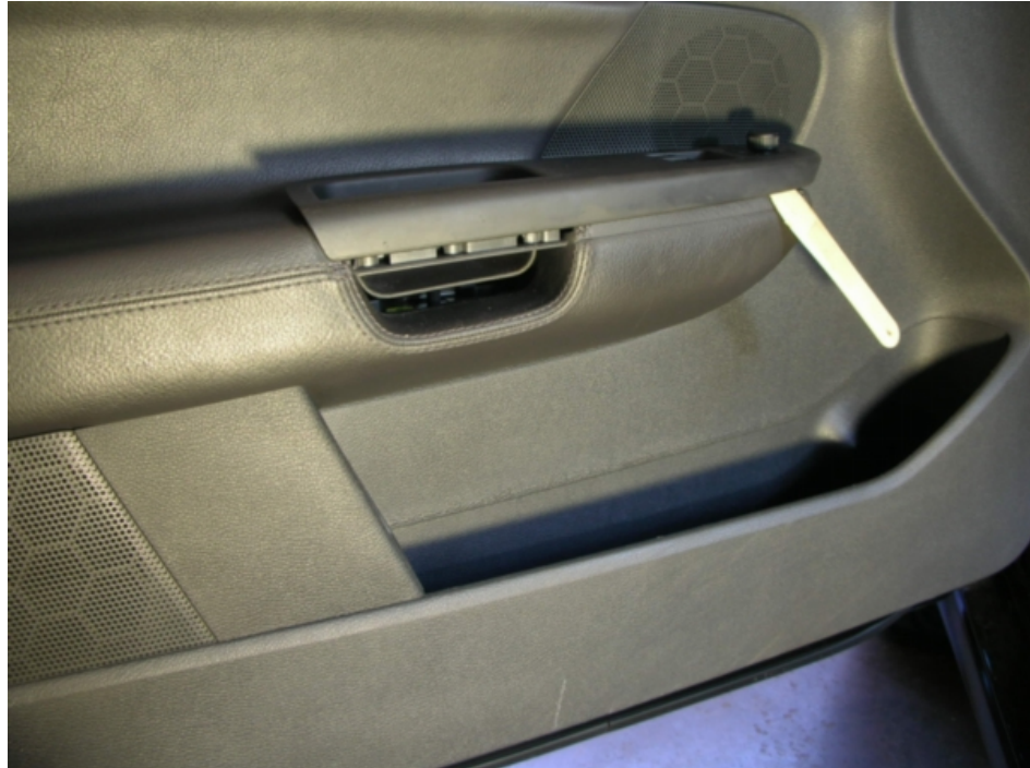
clip locations on the rear and the edge farthest from the door card
