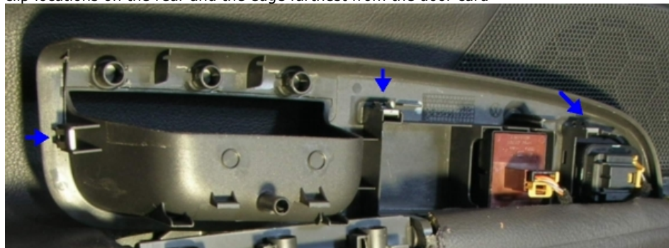
clip locations on the the edge closest to the door card
