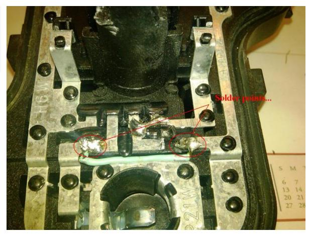
Finally, you're ready to add in the bulb socket. Take the trimmed bulb socket, and put it in the OEM assembly center bit again. Solder the two wires coming from the bulb socket (green and black in this case) to the two metal tabs on the plastic risers. It should look like this when you're done.
