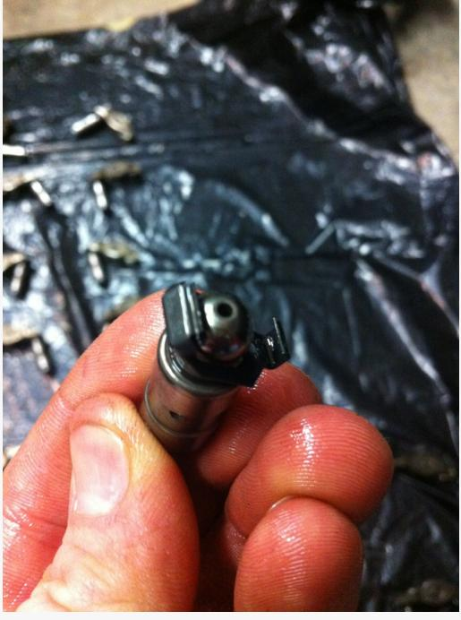
Keep compressing it until you can compress the lifter without the assistance of the paperclip. You wont be able to compress it as far but you v compress it some. It may take as many as 10-15 compressions to fully bleed down.
