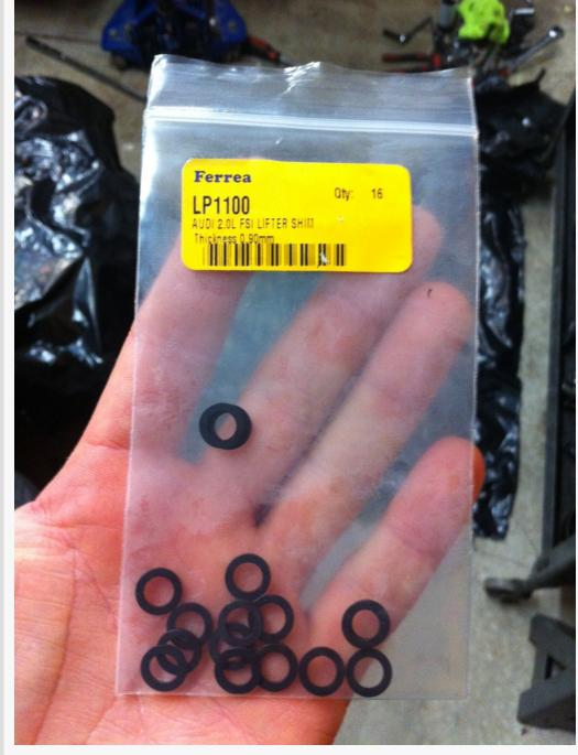
The shims are installed under the lifters in the head. They just drop into place:
