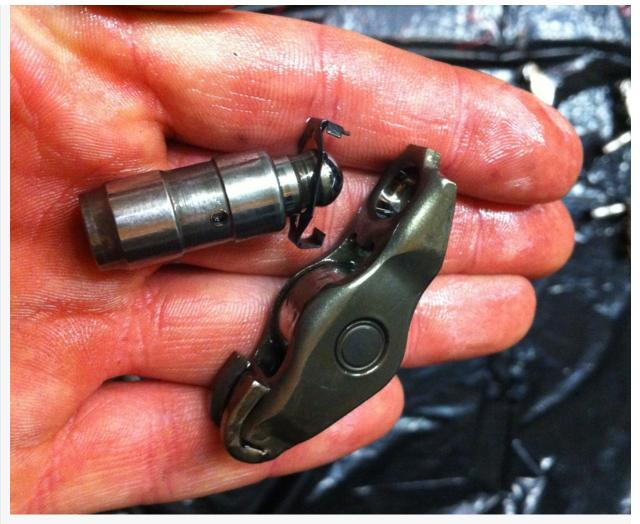
To bleed the lifter, a paperclip can be stuck down the top of the lifter to unseat the check valve inside. It may take a pit of poking around, but it the lifter can be compressed.
