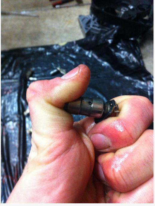
The reason i'm bleeding these down is to make sure that my valves wont be stuck open due to retained oil pressure when I get my lifter shim
