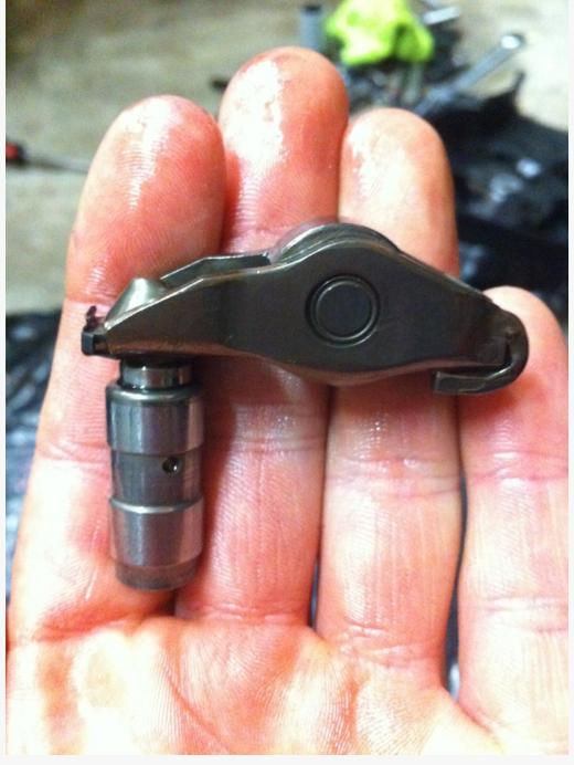
To separate the lifter from the arm, pull down on the tab that holds the lifter on, on the side closest to the lifter itself (left side of this picture)
