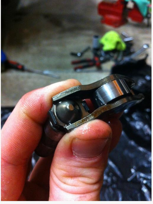
Once you pry down on the tab, the lifter will separate from the arm:
