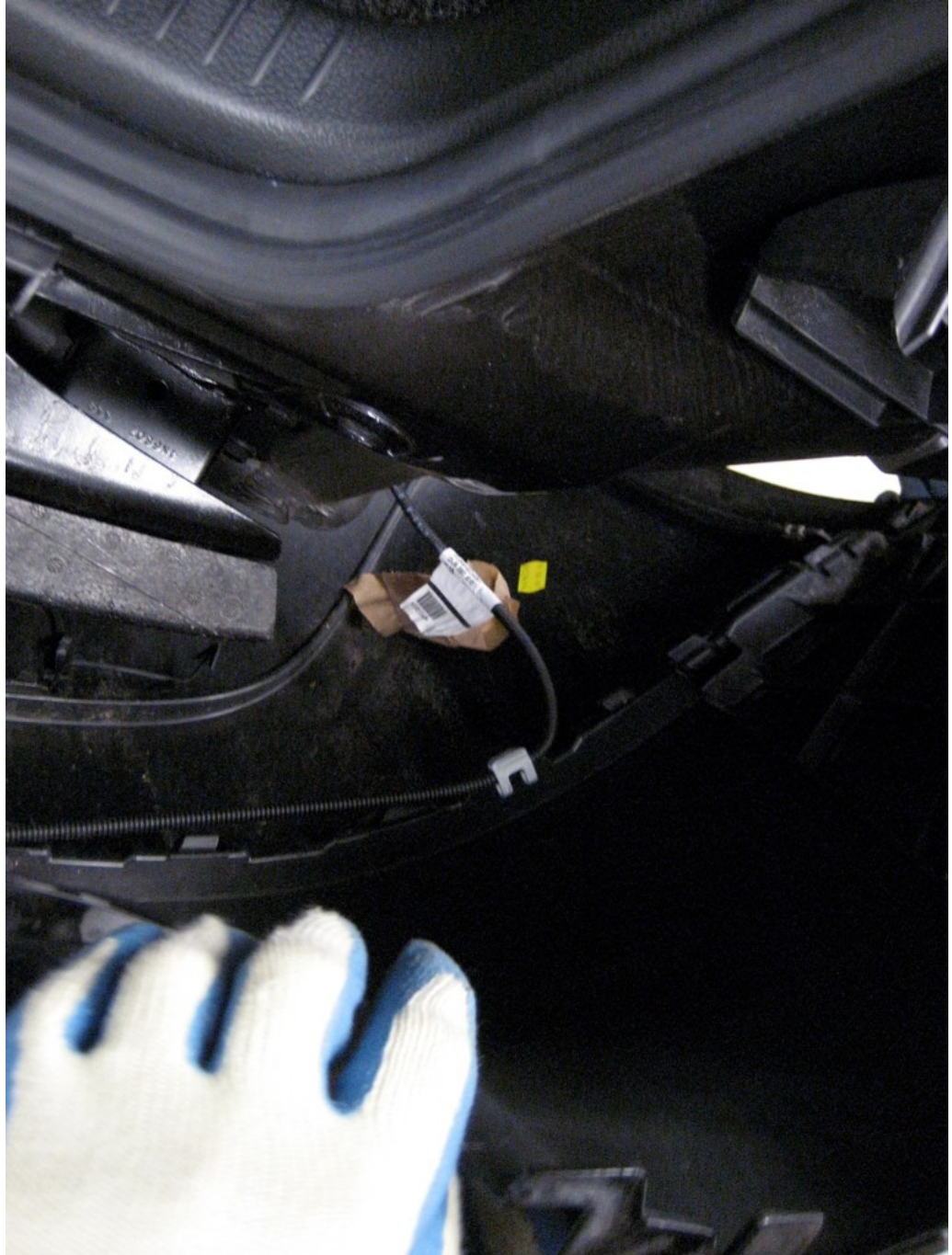
Step 5: pull off cover - give a pull, you may hear a popping sound, that's ok
