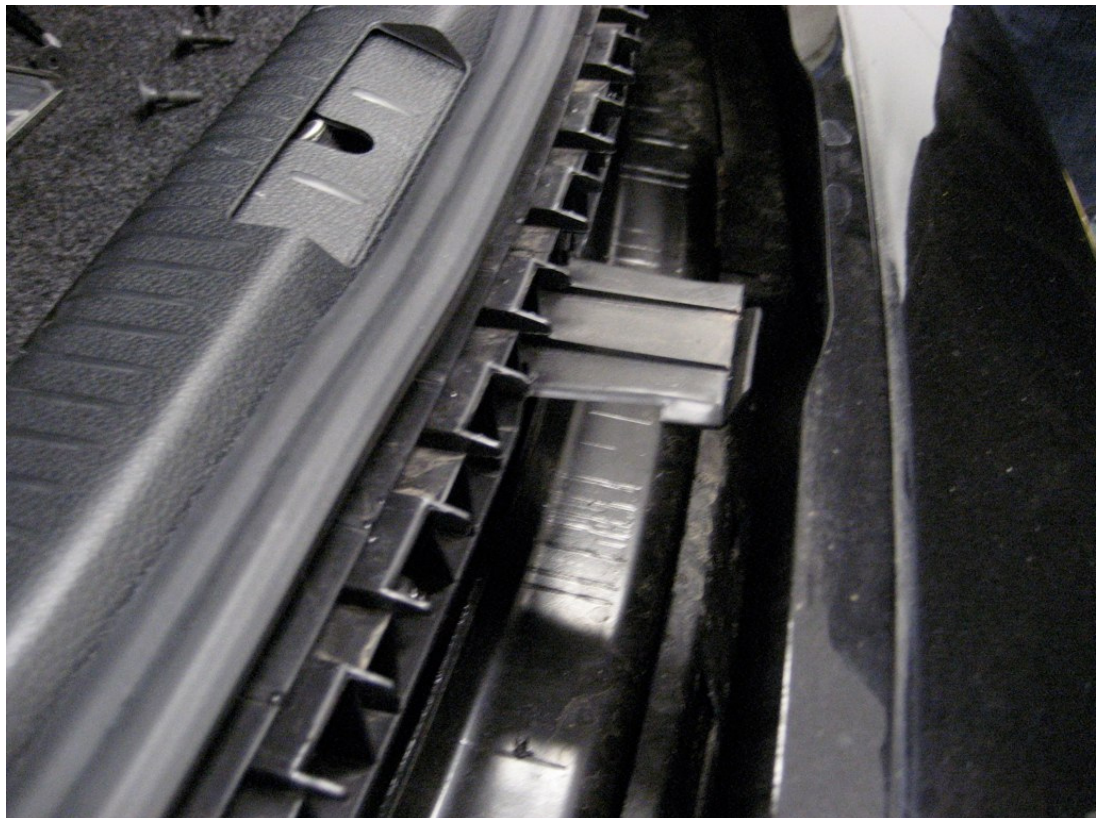
Step 6: Separate the GTI cover top from the bottom:
