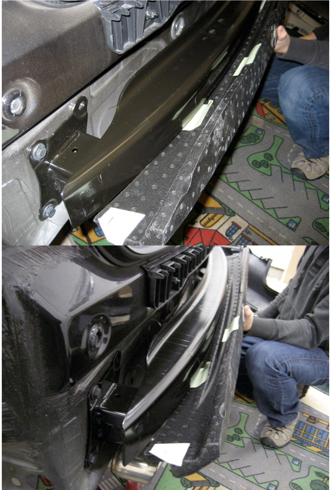
Step 10: slide on the R32 bumper cover: There are "channels" on the both sides that the top cover support plastic will slide into.
