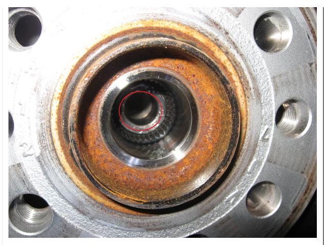
Pound it out enough that you can grasp the axle from the rear and pull on it to tilt it toward the front or rear. I couldn't completely remove it so I left it partially near the end of the wheel hub but it gave me enough remove to remove the 4 triple square bolts to remove the wheel bearing/hub.
