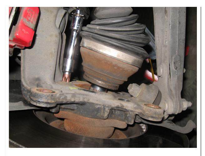
5. Remove the 2 brake caliper mounts held on by 21mm bolts. Once you get the two bolts off, secure the brake calipers so they aren't hanging by the brake line. I used a bungee cord to hang it from my springs.
