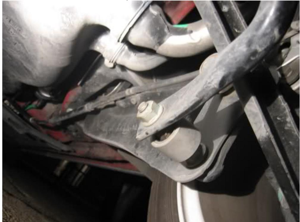
This is where the m10 Triple Square come in. You can use an extension, over the lower control arm to make it easier. be careful not to strip the bolt. (where the spring sits)
