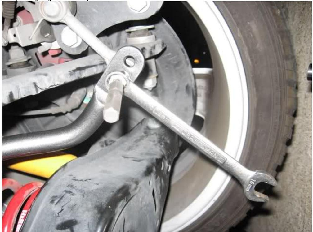
Now at this point, just repeat at putting the bushings on with the m10 triple square and the extension as well for max use.
