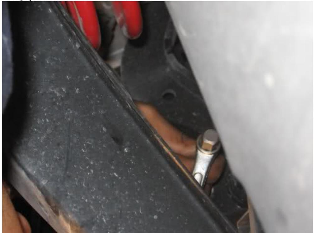
For the H&R there are no new brackets provided. you can use the flat head screw driver to pry off the brackets from the stock bushings. and just slide them over the new bar.
