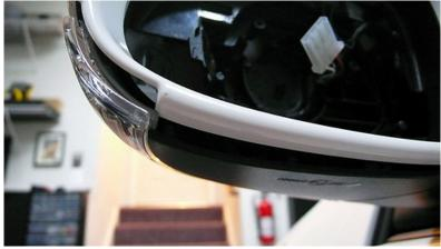
Once the housing is removed, squeeze these tabs to pull/slide out the plastic strip.
