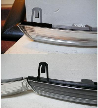
Tilt mirror up using controls until there is a gap:
