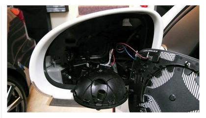
Unplug these. Don't tug too hard. The one with the connector/adapter is a bit tricky. Remember the positive and negative wire locations on the mirror:
