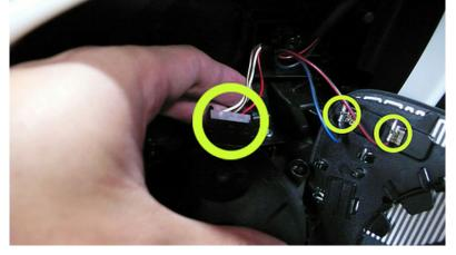
Here is the first tab that connects the side mirror lens to the mirror housing. You'll need to untab this. I used an angled probe, others use screw drivers. Just take your time.
