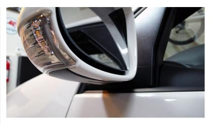
I used a screwdriver wrapped in cloth to gently pry the mirror off. Slip it under the gap. Just don't rush here. You don't want to scratch your mirror housing or break anything behind the mirror. It's not that hard.
