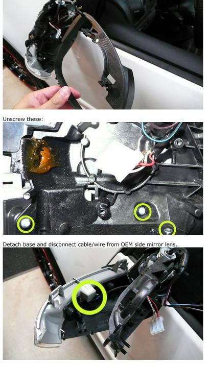
Connect new side mirror lens or side mirror housing. Start reassembling side mirror in the reverse order:
