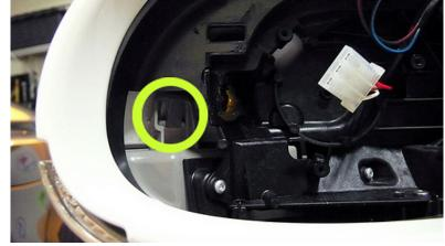
Inside that hole is the second tab. It's a bit more trickier. I used an angled probe for this. Some use screwdrivers:
