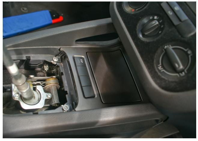
replace the ring if yu didnt break it to badly upon removal or use a zie tie to hold the gear knob in place:
