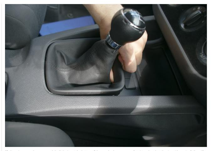
lift the gaitor upwards so yu reveal the little ring at the bottom of the gear knob. squeeze, pull, twist and yank at the ring with a pair of pliers till yu pull upwards on the gear knob to remove it:
