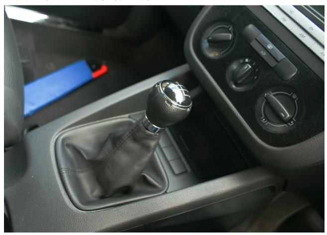
put your thumb under the front side of the gaitor and pull upwards. yu will feel a lip/gap where yu can put your thumbs between and pull! it helps to 2 thumbs under but it had to take a pic at the same time: P:
