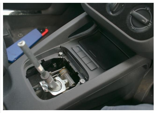
lift up the ashtray and simultaniously pull outwards. yu can wiggle it to get the top edge free as its a bit wide and can get stuck sometimes :) does much to release it! at this point remove both the cigarette lighter/12v plug connector and the ESP connector and lay them to the side. remove the completely:
