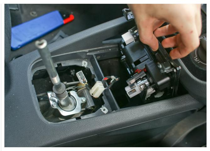
at this point if yu have a full ashtray to replace it with (as i did) yu push the ashtray back in and as with the removal yu give it a wiggle to get the ledge located. plug in the 12v and the ESP connectors and line up the bolt holes. (if yu only have the top plates then splitting them isnt the hardest ever. should be fairly easy to notice the clips yu have to unclip):
