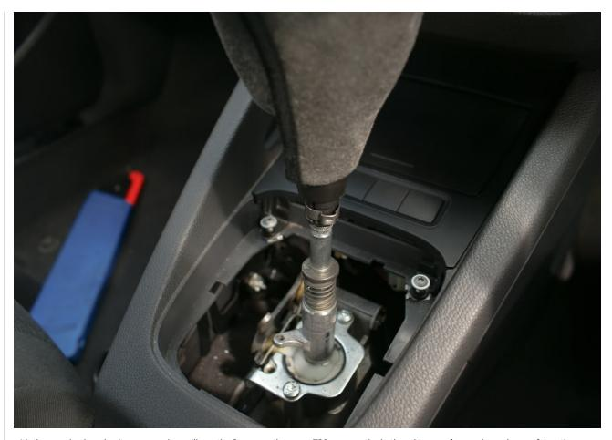
with the gear knob and gaitor removed yu will see the 2 screws. these are T20. unsrew the both and keep safe.. as always be careful as these scre go deep into the depths of your car:
