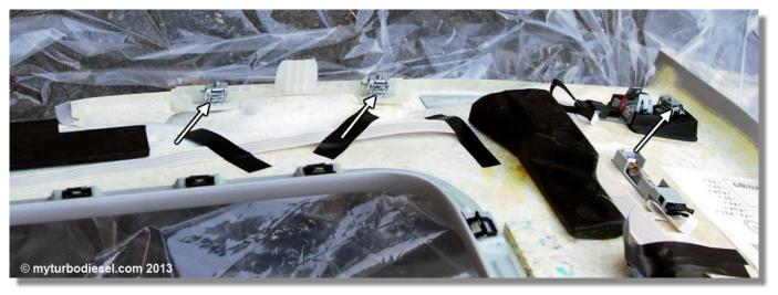
My new headliner had 4 V-clips where the old one used 4 deformable brackets. If your new headliner is like this you only need 10 of those brackets instead of 14. Make sure the holes on the roof are empty for the new clips.
