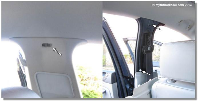
Remove the c-pillar trim. Remove the airbag tag and the torx bolt underneath it. There are a number of hooks along the top which you have to gently pry out. Don't pry against the inside unless you can see the back because the side curtain airbag and radio wiring is behind this trim!
