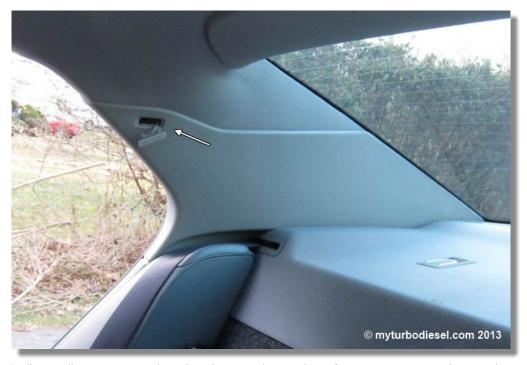
C-pillar installation is easier without the side seat cushion in place. If you want to remove it later, might as well remove it now. It's held with 1x 10mm nut at the bottom of it. Just press the seat bottom corner back as far as it'll go and you'll see the 10mm nut. Then pull the side cushion up to release the hook at the top. During installation, make sure the hook at the top is engaged in the body.
