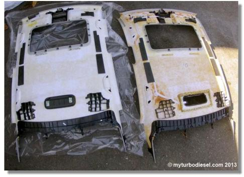
If you wish to reupholster the old one, use a stiff brush to scrape off all the foam on the backing or else the new fabric won't stick well. This is why regluing the old fabric won't work. Make sure to read the instructions on any contact adhesive you use - you normally have to spray both surfaces, let it dry, and then stick it on. I typically use 3M super 90 adhesive.
