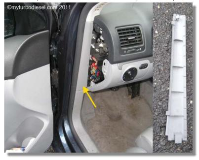
Use a pick to pry out the plastic airbag badge. Remove the T25 torx bolt under the badge. Gently wiggle-pull the trim up and out. Remember to wash your hands a few times during this procedure because the back of all the trim panels will be really dirty.
