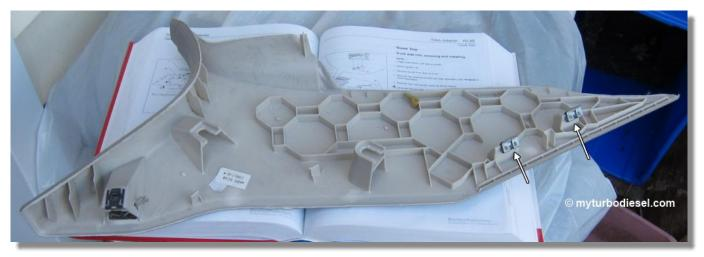
Remove the rear dome light. Its wiring is attached to the headliner so you can remove it now or after the headliner is off the car. If you're going to be doing a lot of headliner bending I'd just remove it now. Pry off the cover and there are 2 hooks at the rear of the light that hold it in place (white arrows). Release the hooks and the plug underneath (visible in next picture).
