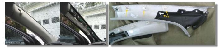
Remove the b-pillar trim: Remove the airbag tag but first note the torx bolt underneath it - it's different so set it apart from the others. Slide the seatbelt adjuster to the top (if it was at the top before you can't see the torx bolt). Use your trim removal tool to pull/pry the aft edge-bottom of the trim towards the rear of the car (there's only 1 snap plug indicated below). The trim then comes down. Let the trim hang off the seatbelt as there's no need to remove it.
