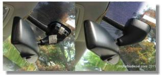
Here is how the mk5 Passat mirror looks. The trim doesn't match up because in this case, the mount was glued below the original spot. Also shown is the headliner trim on the Passat. The hole on the trim covers should match up against this and help hold it in place.
