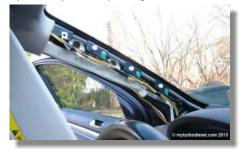
For ground, I soldered together the ground wires for the rain sensor and mirror and ran a single thicker wire back to the fusebox area. I stuck the ground wire under the 13mm nut for the dashboard support (yellow arrow). Yes it's not pretty but I'll never see it again and it's bare metal. If you dig a little more there are some grounds under the overhead lights (next few pics) but make sure it's not on paint or else it won't be a good ground.
