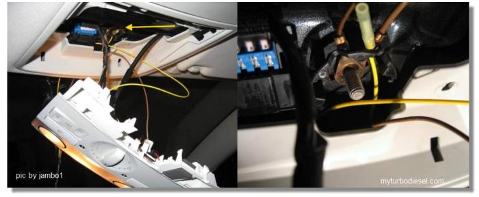
Pass the wiring through the headliner trim. The mirror wire should longer. In this example, the wiring was pretty tight so you may want to leave them about 0.7-1.0 cm longer than shown and stuff any excess under the headliner. You can also see the difference in color between the beige trim and pearl grey headliner. After installation I never looked at it again so the color difference isn't really noticeable.
