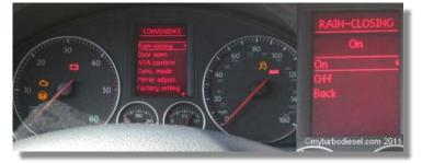
Because you disconnected the battery, the steering assist and ESP are reset and will show the above lights. This should be resolved through regular driving. You also need to reset the one touch windows by raising and then pressing up again, then lowering, and pressing down again. If you have power seats, do the same thing with the range of motion to reset the memory. If there is a problem, see <u>1000q</u>: steering wheel adaptation reset.
