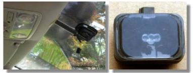
Slide the new mirror up on the mount rails until the stop. Plug in the wires and snap the trim covers on. Reconnect the battery and headlight switch. You can leave the covers off if you wish to test the sensors first. Note that the black painted area matches the edge of the mirror base trim.
