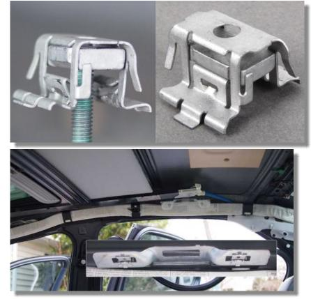
Insert a screwdriver or your key in the slot on the fusebox cover and pop it off. Remove the trim strip shown below. Press the door seal back a little and gently pull to release the clip at the top. Lift it up and out.
