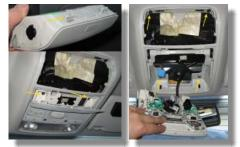
Loosen the headliner by removing the sunvisors and front grab handles. This makes it much easier to route the wiring. Use a pick to pop their covers off and remove the T20 screws holding them. If you choose to not loosen the headliner, use a wire snake (a bent coathanger) to push the wiring through.
