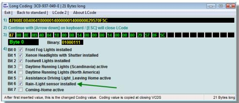
The rain sensor should now work! The intermittent position on the wiper stalk is now auto-sense. The dial which used to be intermittent wiper speed is now sensor sensitivity. If you wish to enable rain closing, see <u>1000g: rain closing function</u>. If you do, you'll see this option on the convenience menu.
