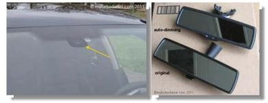
The rain-light sensor controls the auto headlights and auto wipers. It shines infrared light out and looks for a reflection. Therefore, the sensor must have a clear view outside and be mounted within the swept area of the wiper arms so that the glass over the sensor will be cleaned. The mount for the sensor is also the mount for the OEM auto dimming rear view mirror. The base of the auto-dimming and non-dimming mirror are completely different as seen above.
