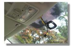
When installing the sensor on the mirror, make sure the jelly pad is clean. There should be no air pockets between the sensor and windshield. For some reason, all of the sensors I've seen with this part number (version r) have two gaps at the bottom. Once you install it, the gaps disappear. There are a few versions which will work on different platforms so check part compatibility before using any random VW-Audi light sensor.
