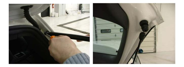
Then use a 13mm wrench to remove the old mounting pin. Install the new mounting pin and the new hatch strut. Repeat for the other side.
