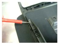
Once separated, you can now remove the outer and inner vents on the left side to make room for the new gauge pod. Simply pull out the outer and the inner is held in by tabs on the bottom, simply pry up on bottom tabs and remove. Install the new gauge pod and reattach the outer trim for the center vents. If needed, glue the plastic welded pieces back to their original state.
