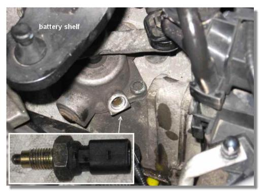
Another method to refill the gear oil is to use compressed air to force the fluid into the fill hole. It's not possible to use a funnel on many cars so I originally made this for my Audi and on other cars where the fill hose has to go up. It can also quickly move the fluid into the transmission if you're using a small hose through the reverse switch hole. The basic idea is that you use compressed air to force fluid out of the container and through the hose.
