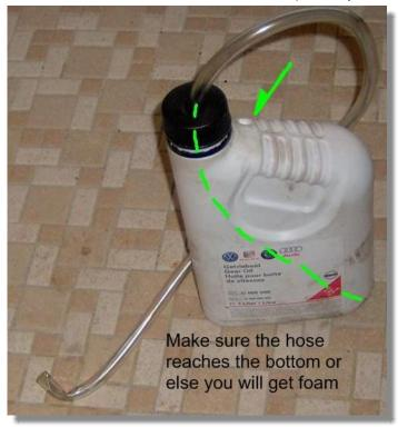
Regulate the air pressure down to a reasonable amount. If the air pressure is too low the fluid won't move and if the air pressure is too high the bottle
