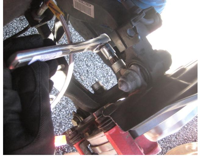
5. Remove the carrier and remove the old pads from it. Set it aside.
