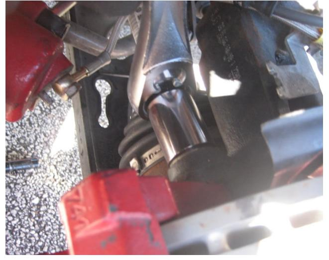
5. Then remove the carrier and the screw that holds the rotor on, remove the old pad from the carrier
