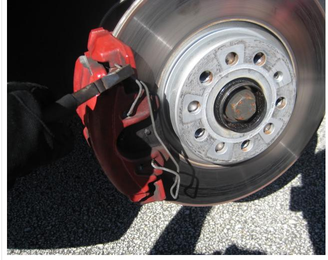
2. Remove the black plastic caps covering the bolt that hold the caliper on. Using a 7 mm allen wrench, remove both of the bolts.
