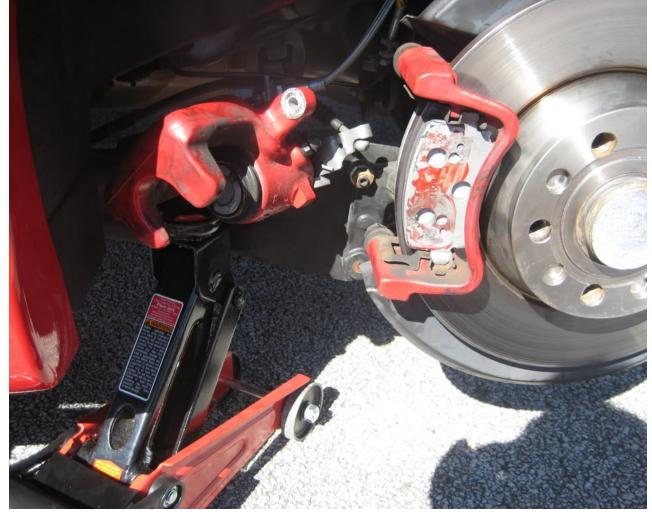
4. Remove the two bolts holding on the carrier using an M14 twelve point bit.
