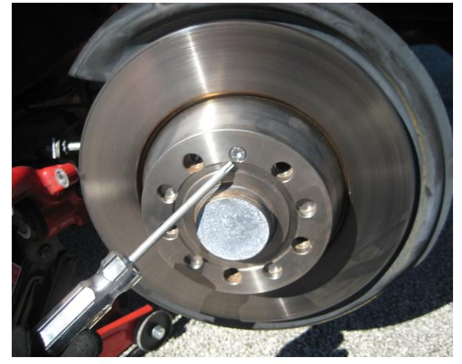
6. Replace the rotor and the screw that holds it on, then lightly grease the carrier bolts and bolt the carrier back on
