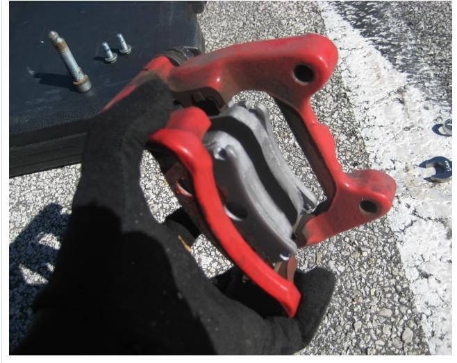
9. Replace the rotor and bolt the carrier back on, place some grease on the carrier bolts
