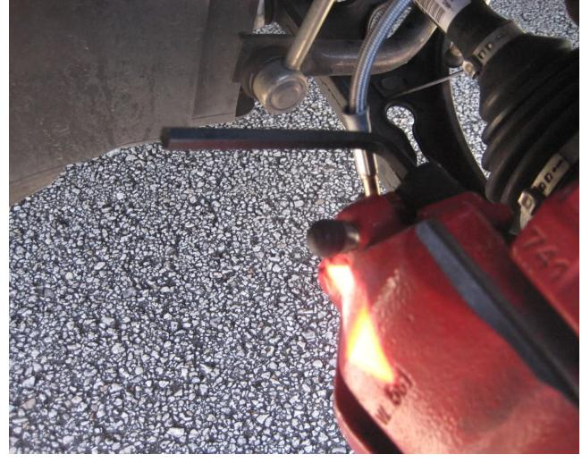
3. Remove and secure the caliper so that the lines aren't stretched
