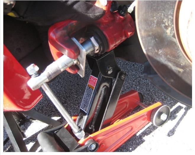
11. Slide the caliper onto the carrier and bolt the caliper back on
