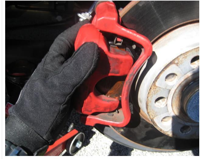
12. Check all of the bolts to make sure that they are tight. Make sure that your lines are not leaking at the fittings, and make sure that the rotors clean. You can spray them with Brake Cleaner to make sure, but do not let the brake cleaner touch the brake pads
