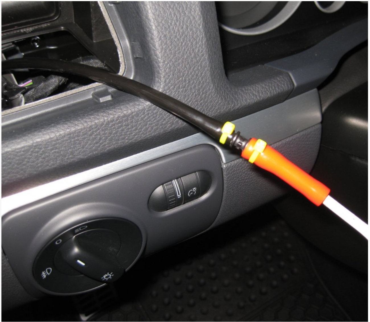
You can see the 3 yellow tie wraps where I ran the boost hose through the proper cleanest channel:
