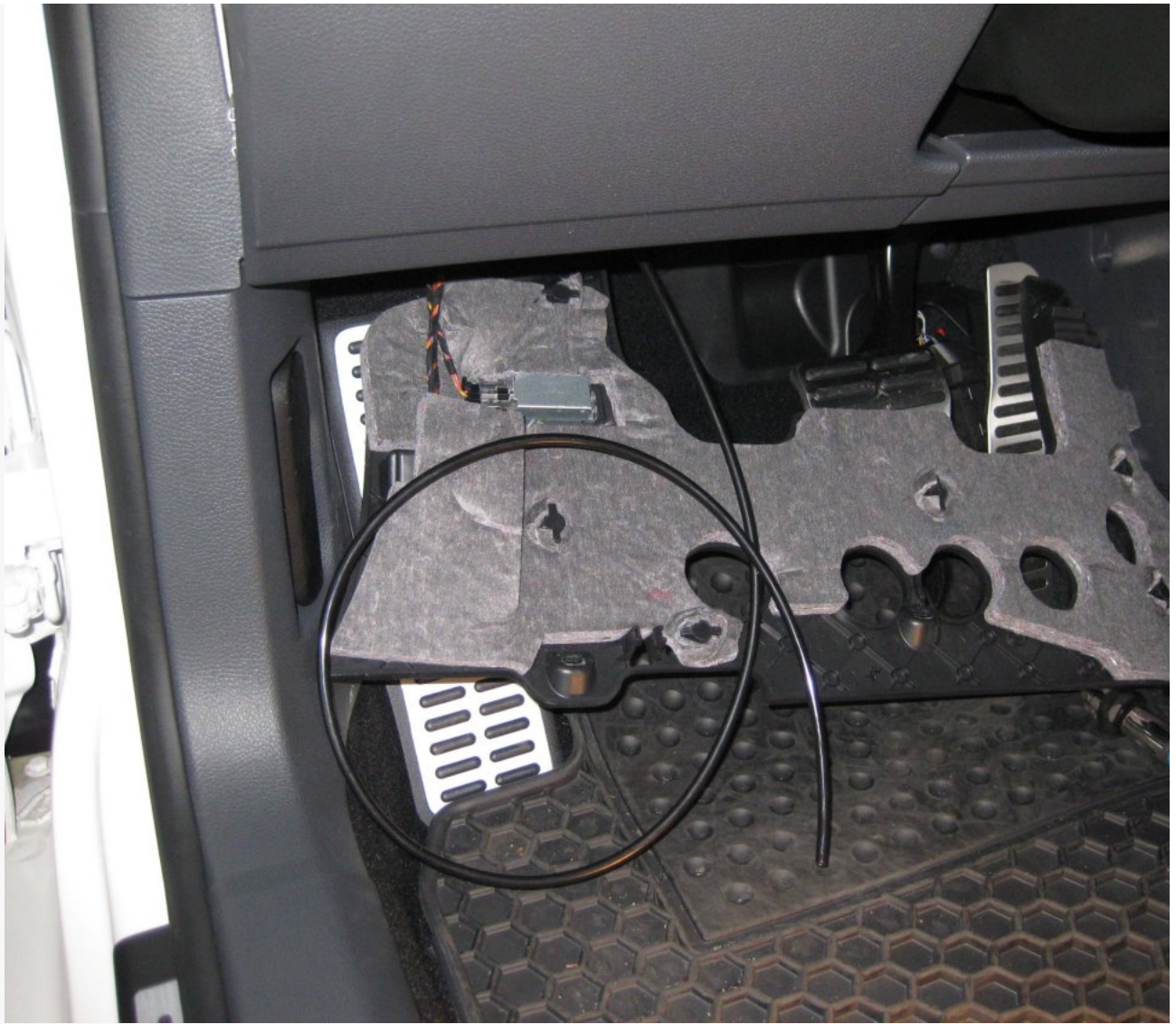
Showing the parts off the TSI which had to be removed to route the hose properly. The TSI could be considered harder than the FSI since you also airbox:
