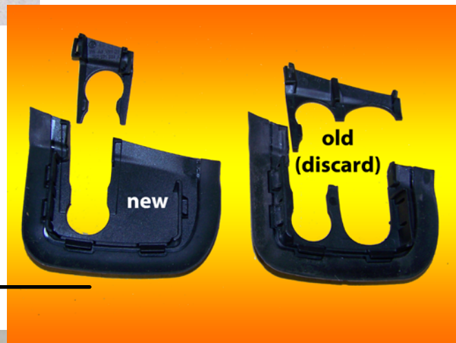
Water tray original retainer and replacement blockoff.
