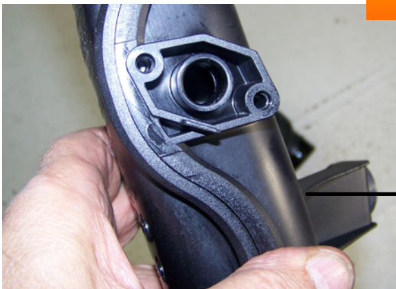
Pressure sensor hole in air duct. Install sensor carefully to avoid damaging the sensor seal.
