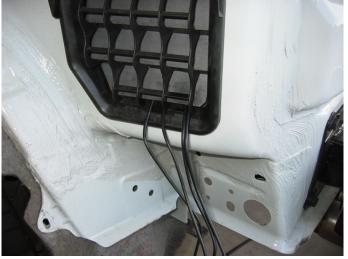
40. Pull the wires up through the driver's side rear well (behind the brake light area).
