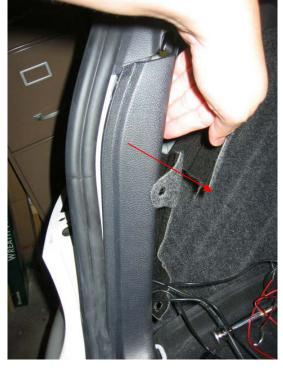
14. Use a T-20 driver to remove the screw that's behind the panel in Step #13.
