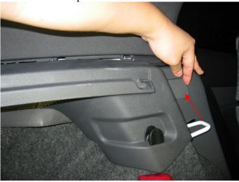
16. Use a T-20 driver to remove the screw behind the panel in Step #15. Pull the panel outward as arrowed below.
