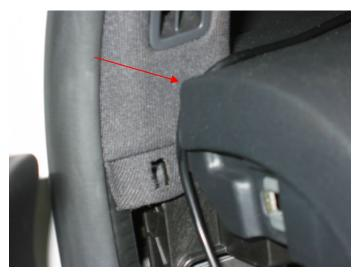
26. Push the hood release panel outward, and feed the wire through the panel, in the direction of the arrows.
