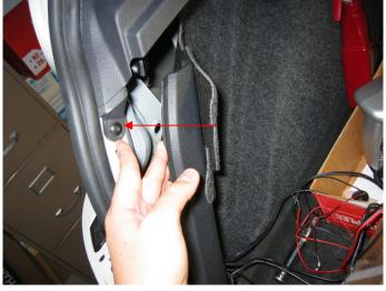
15. Remove the panel arrowed to below.
