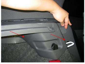
19. Here is the pic of the panel removed in Step #18. Arrowed to are the 3 plastic retaining posts that hold the panel piece on, in addition to the screws that where removed in Steps #14 & 17.
