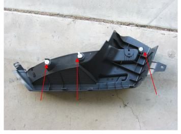
20. Using something dull, pry the door foot panel upwards to start unclipping the door foot panel. Be careful not to damage the panel. Remove all the clips along the door. There are about 5 or so clips (I don't remember exactly)
