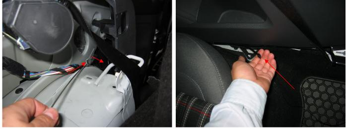
29. Tie the display wires and back-up light signal wire on the snake (left) and duct tape it real well (right)
