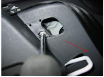
17. Use a T-20 driver to remove the screw arrowed to below.
